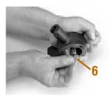
7. Install integral oil pump inner element on drive shaft, aligning round key on drive shaft with round keyway on inner element and square key on drive shaft with square keyway on inner element.
