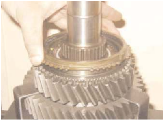
8. Lubricate the 3rd gear synchroniser flange and then fit the synchroniser ring.
