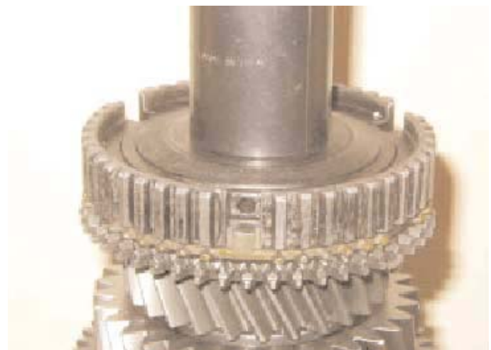
19. Heat the 5th /6th -speed synchroniser hub to 85; Centigrade and then install it, boss downwards, onto the mainshaft. Ensure that the large slots on the synchroniser hub align with the large shoulders on the synchroniser ring. Press the synchroniser hub until it is fully seated.
