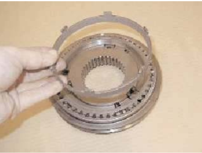
5. Remove the synchroniser friction ring.
