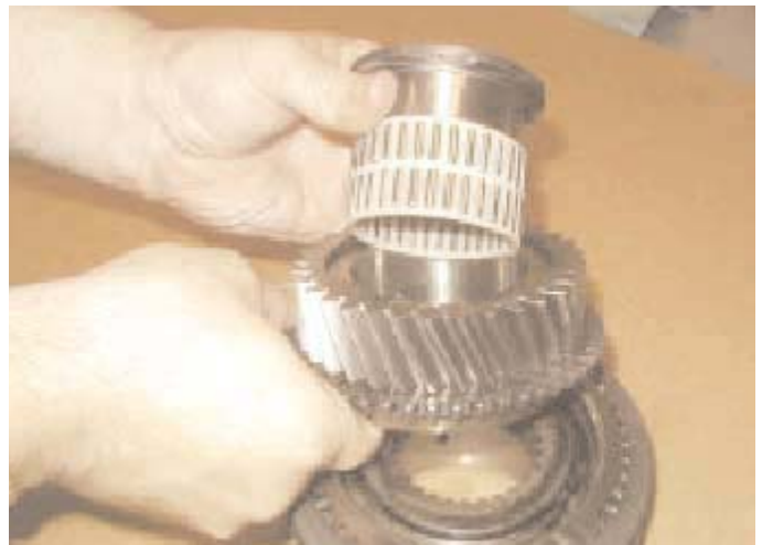
15. Place the assembly on to a suitable work surface, 4th speed gear, uppermost. Remove the bearing sleeve, needle roller bearing and 4th gear assembly
