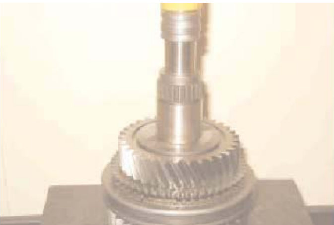
14. Using a suitable press or puller support the mainshaft assembly underneath 3rd speed gear. Note: It is imperative that the flange, which is part of the mainshaft, does not foul the press or puller legs as this may result in damage to the mainshaft. Press or pull the 4th speed gear bearing sleeve, 4th speed needle roller bearing, 4th speed gear assembly, 3rd /4th -speed synchroniser assembly and 3rd speed gear assembly off. Remove the 3rd speed gear needle roller bearing from the mainshaft.
