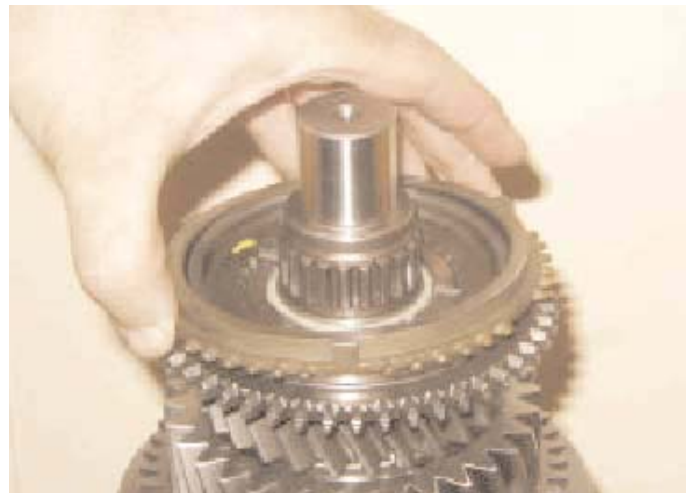
18. Lubricate the 5th gear synchroniser flange. Fit the synchroniser ring.
