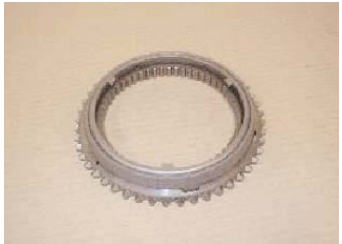
g) Fit the synchroniser friction ring on to the synchroniser flange ensuring that the tabs on the synchroniser friction ring locate into the slots on the synchroniser flange.
