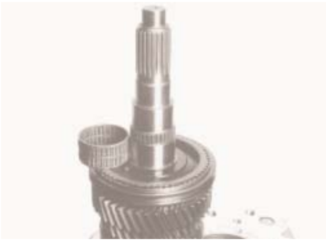
9. Lift off the steel cage bearing, 1st gear synchroniser ring.
