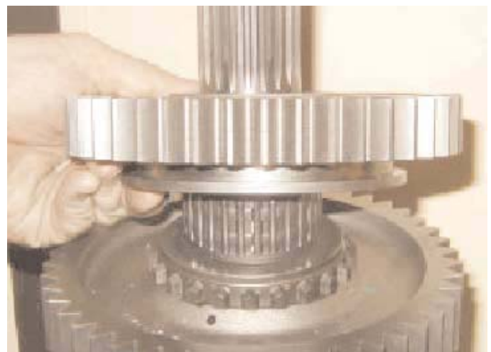
29. Fit the reverse gear needle roller bearing. Lubricate the bearing and then fit the reverse gear, boss down, onto the mainshaft.
