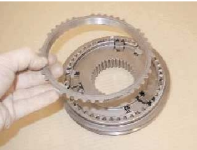
6. Remove the synchroniser ring.
