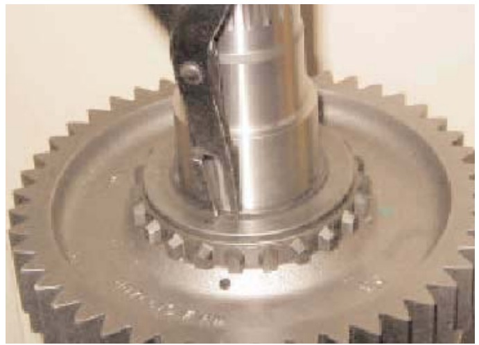
27. From the range of graded circlips select the one which fits into the mainshaft groove with the least amount of free play. Fit the Circlip into the groove taking care not to damage the mainshaft needle roller bearing surface.
