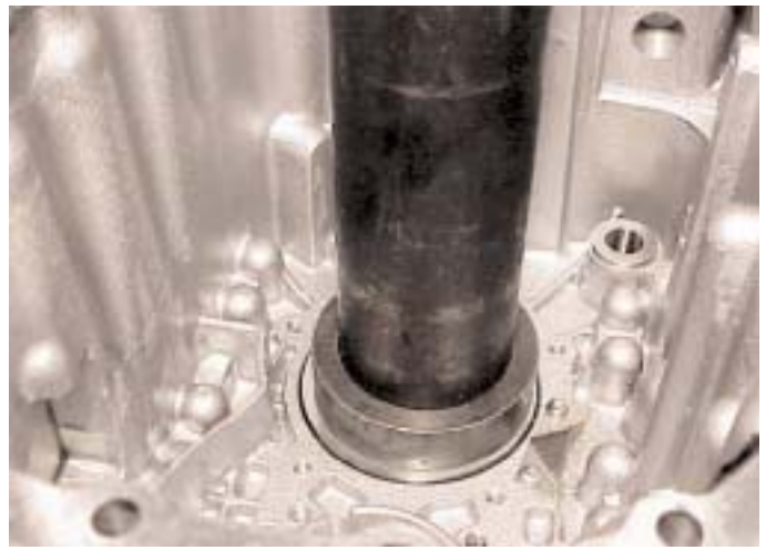
32. Drift out the layshaft front bearing cup using the special tool. Remove the input shaft bearing using the special tool.
