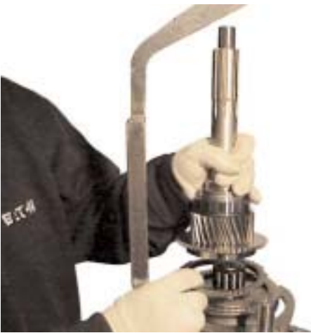
24. Lift off the input shaft with 6th gear flange. Remove the 6th gear synchroniser ring.
