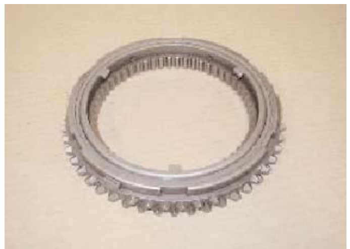
i) Fit the synchroniser ring onto the assembly.
