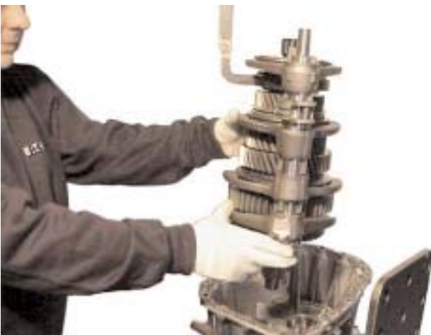
25. Raise the hoist and lift out the mainshaft and selector shaft and forks as an assembly. Carefully lower on to a clean bench and remove the special tool. Separate the selector shaft and forks from the mainshaft.
