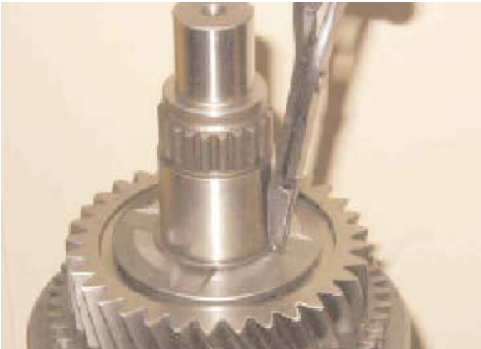
15. Fit a new snap ring into the mainshaft groove taking care not to damage the mainshaft-bearing surface.
