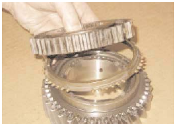
17. Lift off the synchroniser hub and synchroniser ring.
