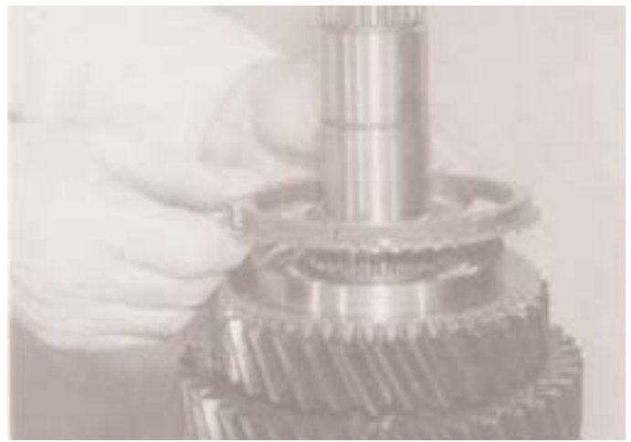
20. Install the 3rd gear synchroniser ring over the flange.
