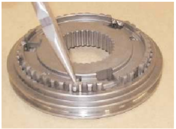
8. Taking care not to lose the balls or springs lift the detent poppets to release the balls. Once the balls have been removed it is possible to remove the detent poppets and springs.
