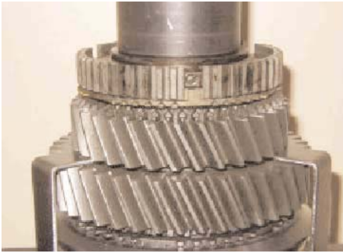
9. Heat the 3rd /4th -gear synchroniser hub to 85; Centigrade. Fit the synchroniser hub over the splines on the mainshaft ensuring that the large slots in the synchroniser hub align with the large shoulders on the synchroniser ring. Press the synchroniser fully home.
