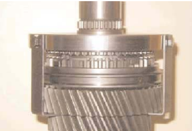
8. To prevent the synchroniser assembly from separating during removal fit the retaining tool. The tool fits onto the mainshaft, boss down, with the three retainers located underneath 2nd speed gear. Adjust the retainers so that there is no free play between 2nd speed gear and synchroniser assembly.
