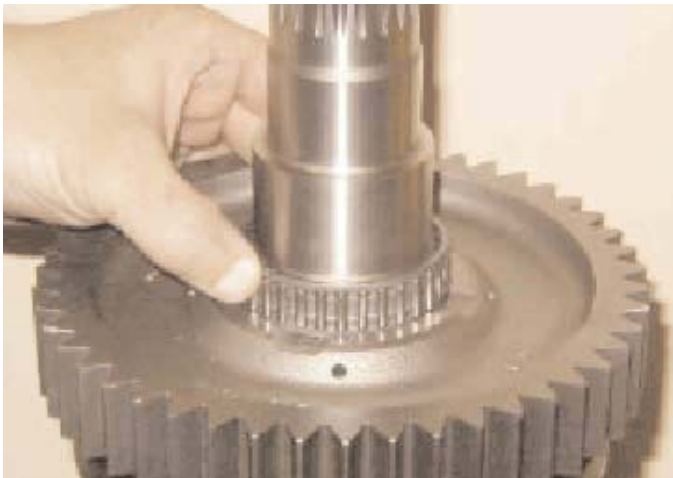
25. Fit and lubricate the needle roller bearing. Fit the 1st speed gear ensuring that the splines on the 1st speed gear engage into the splines of the synchroniser flange.
