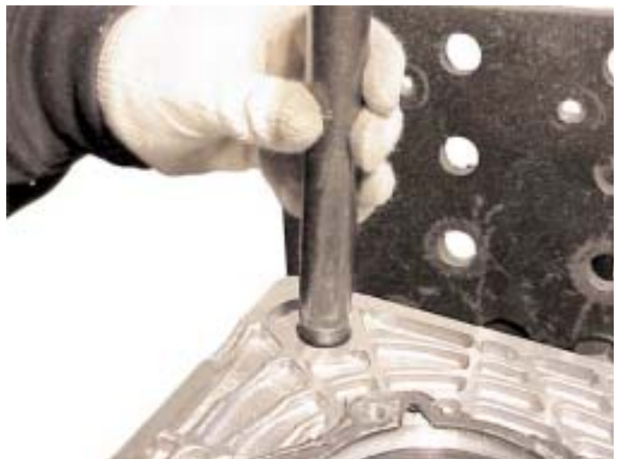
34. Invert the case halves and using the special tool or a suitable (25mm diameter) mandrel drive the selector shaft bushes out of the cases.
