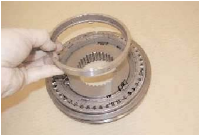
d) Remove the synchroniser inner ring.
