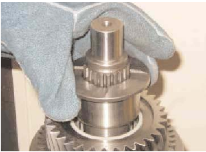
14. Heat the 4th speed gear-bearing sleeve to 85; Centigrade and locate it onto the mainshaft and inside the needle roller bearing. Press the bearing sleeve into position.
