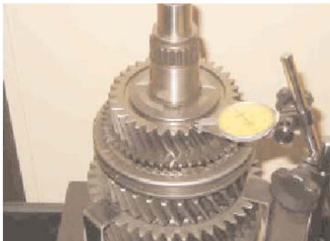
16. Check that the 4th gear end float is within the tolerance stated in the chart.
