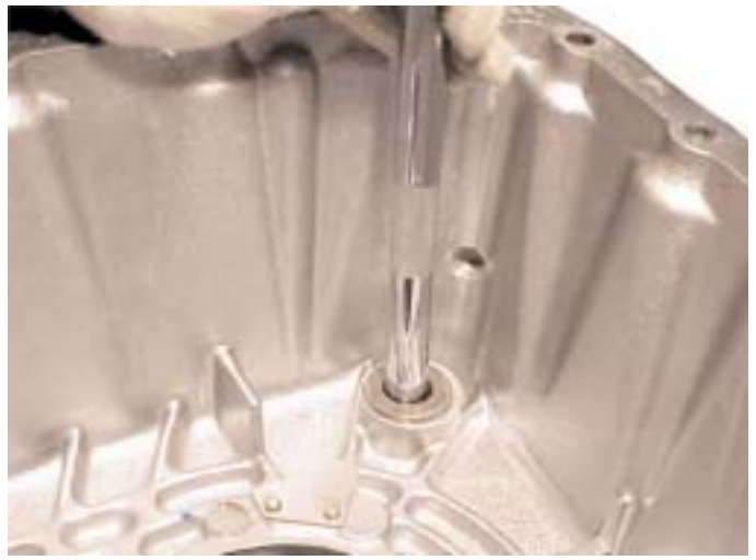
33. If necessary, to renew the selector shaft bushes, drive the selector shaft expansion plugs outwards from the case halves.
