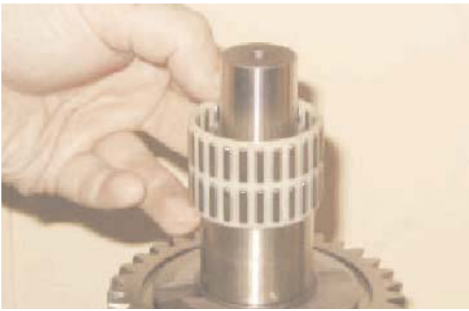
12. Remove the 5th gear needle roller bearing. (On overdrive transmissions this will be 6th gear).
