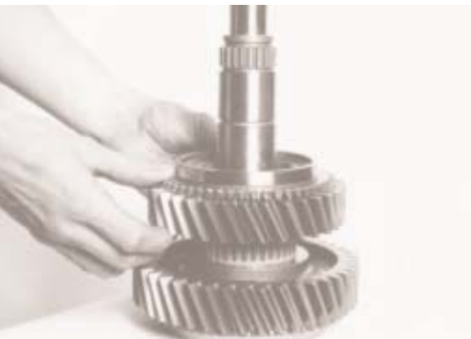
19. Invert the shaft in the vice. Lubricate and install the 3rd bearing and 3rd gear assembly.
