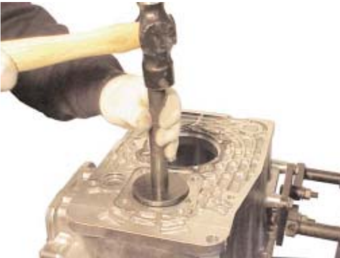
30. Drift out the layshaft rear bearing outer cup using the special tool.
