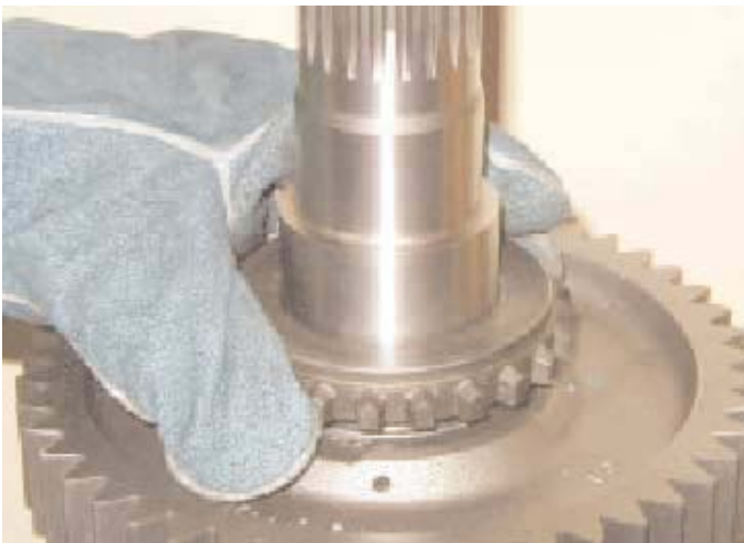
26. Heat the reverse gear hub to 85; Centigrade and then, with the boss uppermost, fit it onto the splines of the mainshaft. Press the reverse gear hub until it is fully seated.
