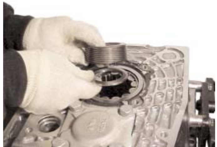
27. Remove the speedometer drive gear or tachograph rotor and the bearing spacer from the rear case half.
