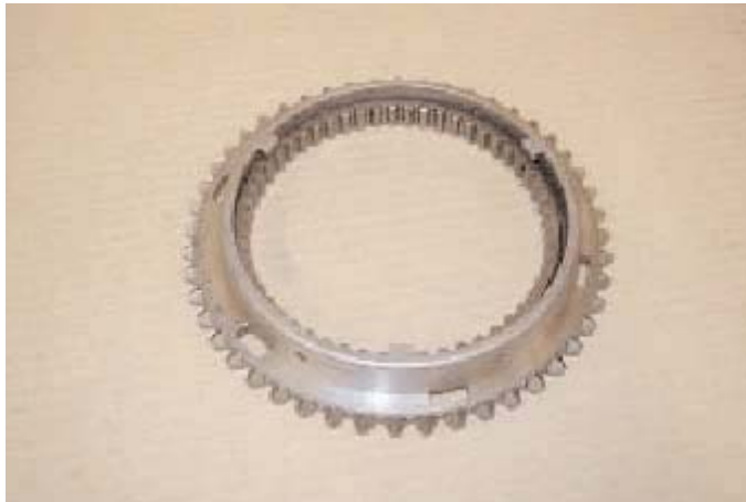
e) Fit the synchroniser inner ring, tangs uppermost, on to the synchroniser flange.
