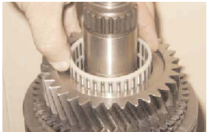
13. Fit the 4th speed gear assembly. Lubricate the needle roller bearing and then install it into the gear.
