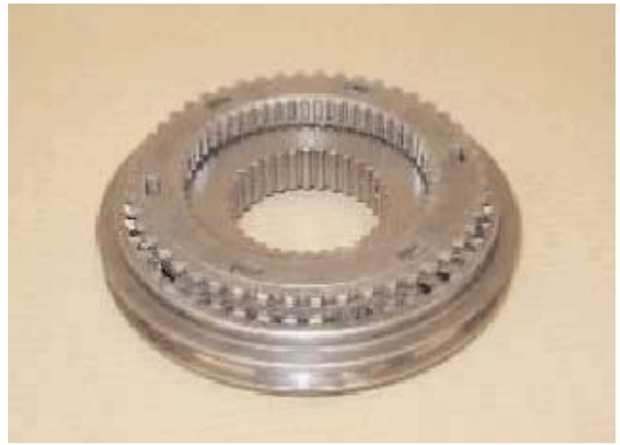
16. Hold the synchroniser assembly down against the bench and at the same time lift the synchroniser sleeve upwards to engage the neutral position.
