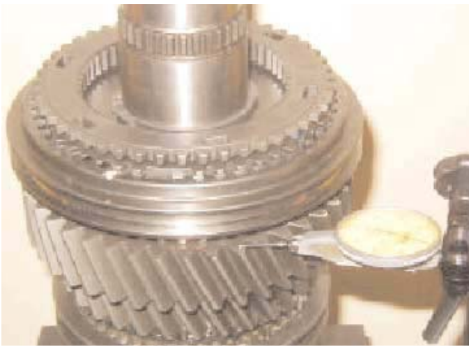
24. Check that the 2nd speed gear end float is within the tolerances stated in the chart.
