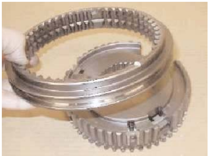
9. Remove the synchroniser sleeve.
