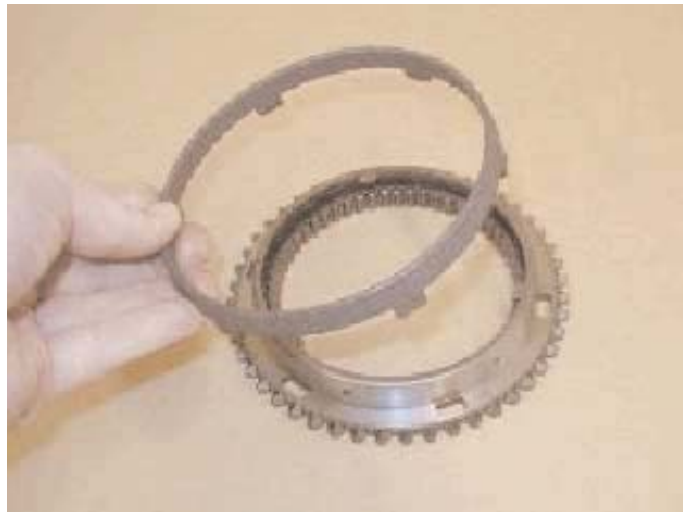
13. Remove the synchroniser friction ring.
