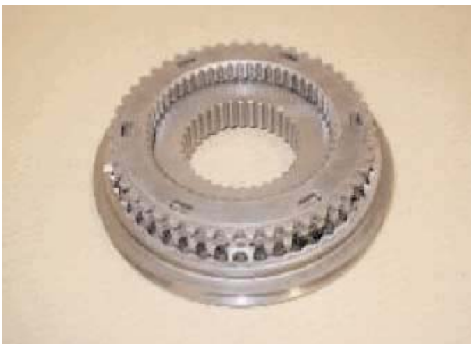
15. Place the synchroniser flange in to position ensuring that the slots of the synchroniser flange align with the tabs of the synchroniser friction ring.
