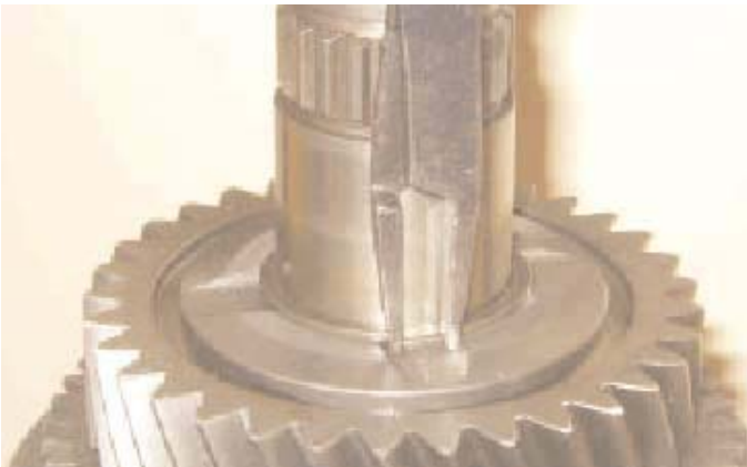
13. Carefully remove the 4th gear-bearing sleeve retaining snap ring.
