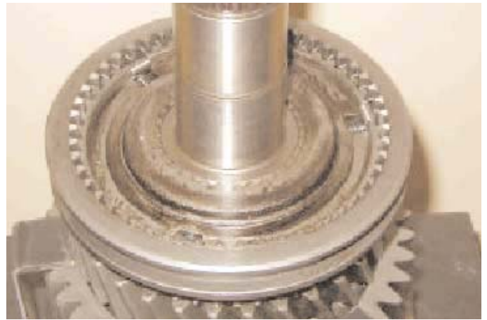
11. Assemble the three springs and plungers into the synchroniser hub. Place the synchroniser sleeve over the synchroniser hub and support it with the internal groove just above the synchroniser hub. Position the three rollers as shown, resting on the heads of the plungers, and press downward on the synchroniser sleeve. This compresses the springs allowing the synchroniser sleeve to centralise in the neutral position.
