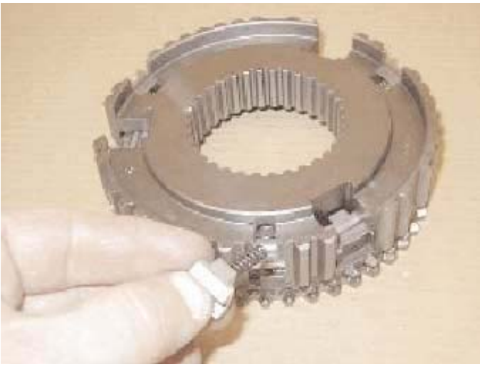
10. If not already removed at step eight remove the detent poppets and springs.
