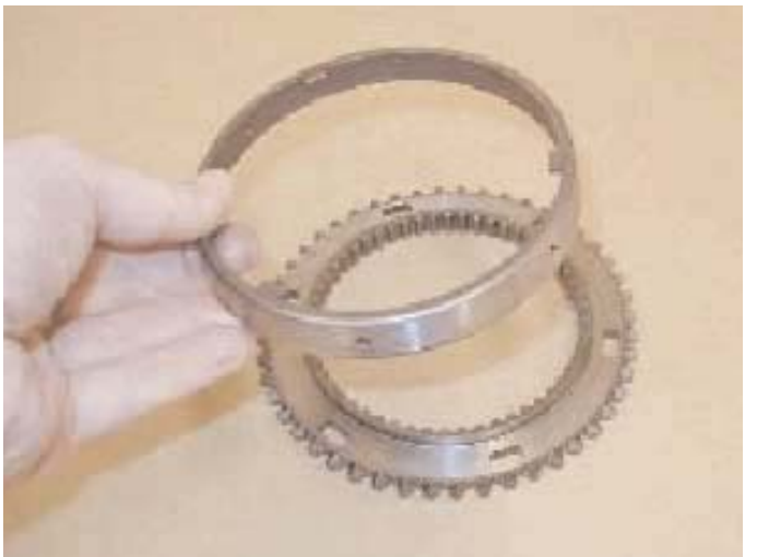
14. Remove the synchroniser inner ring.
