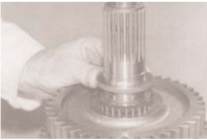
17. Fit the spacer on the standard cylindrical roller or 4 point ball bearing. If integral spacer bearing is fitted the spacer is part of the bearing inner race.
