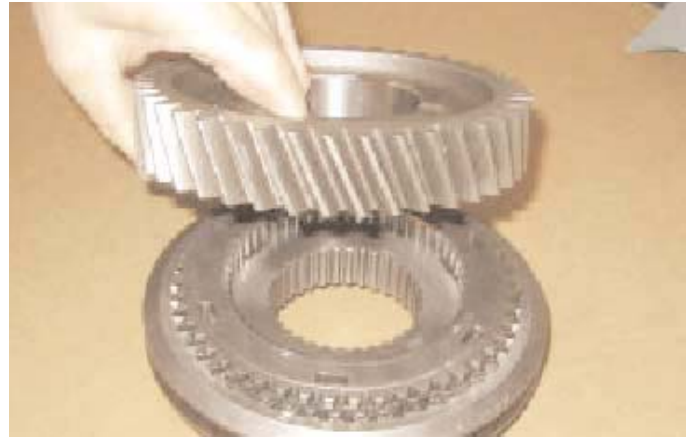
10. Carefully remove the retaining tool and then place the synchroniser assembly and 2nd speed gear onto a suitable work surface. Remove 2nd speed gear.
