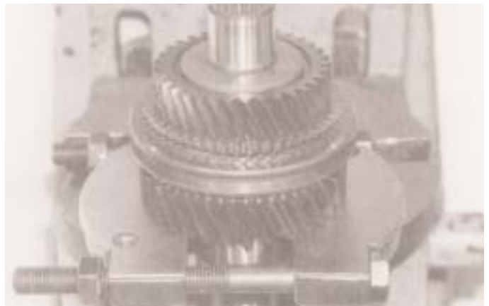
13. Support the shaft on the press under 3rd gear. Note: It is imperative that 3rd gear is supported and that the flange on the shaft does not foul the supporting blocks or press bed when the shaft is being pressed through. Press or pull the shaft through 3rd gear, 3rd/4th gear synchroniser hub and 4th gear bearing sleeve.
