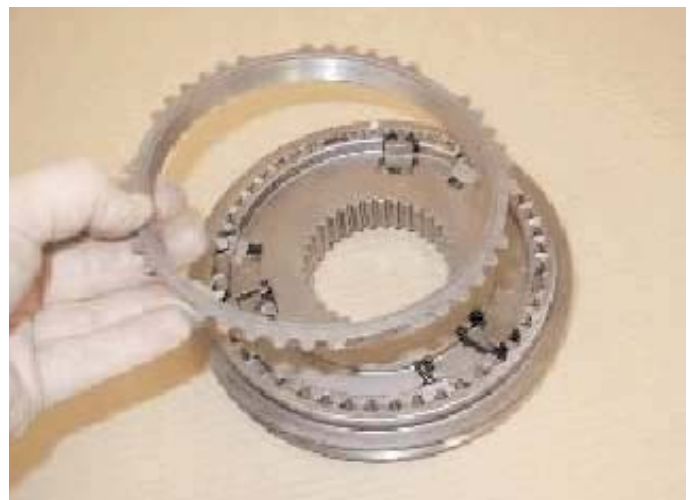
h) Remove the synchroniser ring.
