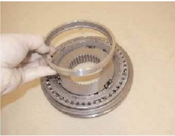
4. Remove the synchroniser inner ring.
