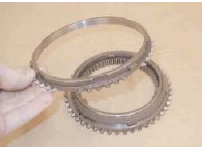
12. Remove the synchroniser ring.
