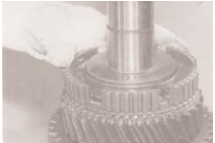
21. Take the heated 3rd/4th gear synchroniser hub and fit it over the splines on the shaft ensuring that the large slots in the hub align with the large shoulders on the synchroniser ring. Use a soft drift or flanged driver if necessary to ensure the hub is fully home. Recheck that the shoulders are in the correct slots
