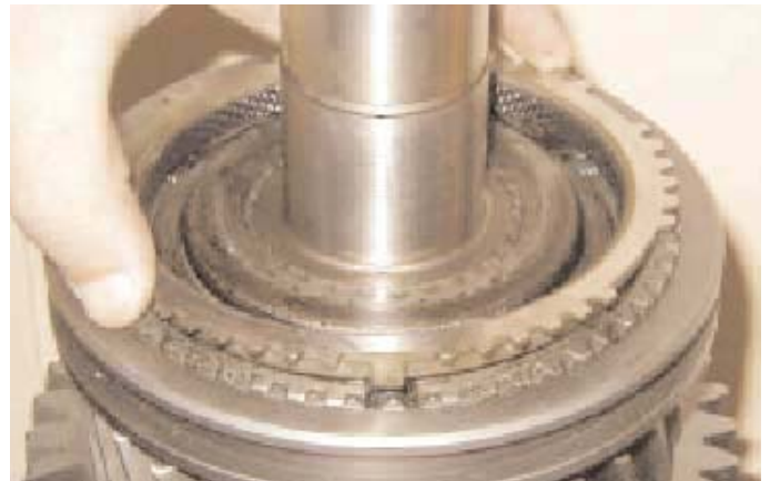
12. Place the 4th gear synchroniser ring onto the synchroniser assembly ensuring that the shoulders on the synchroniser ring locate into the slots of the synchroniser hub. Lubricate the synchroniser ring.
