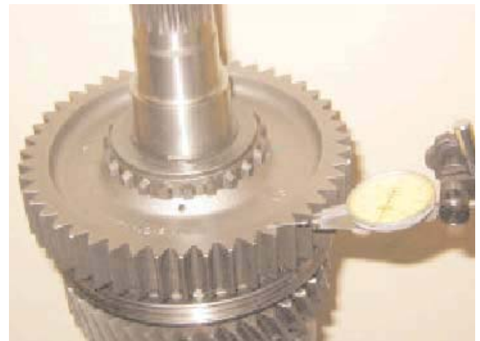
28. Check that the 1st speed gear is within the specified tolerance stated in the chart.
