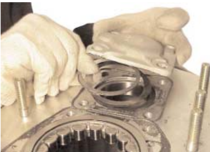
31. Remove the layshaft front bearing retaining plate and graded spacer from the front case.
