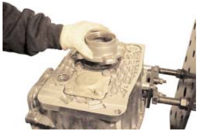
26. Invert the rear case on the stand and remove the capscrews securing the speedometer housing. Note the positions of the different length capscrews. Remove the housing. If necessary drift out the oil seal.
