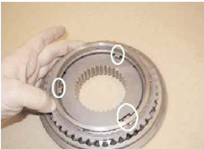
14. Place the synchroniser inner ring in to position ensuring that the three tabs align with the legs of the blocks.
