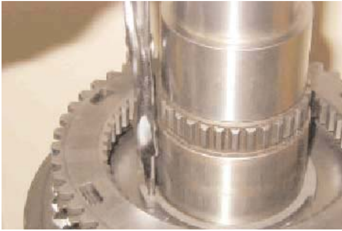
7. Remove the synchroniser assembly retaining Circlip.
