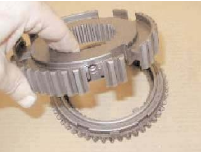
11. Remove the synchroniser hub.
