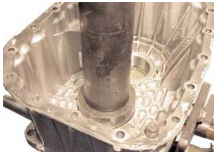
28. Invert the casing on the stand and using the special tool drift out the mainshaft rear bearing. Do not allow the bearing to fall to the floor.
