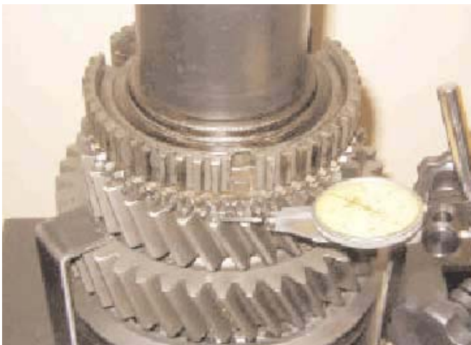
10. Check that the 3rd gear end float is within the tolerance stated in the chart.
