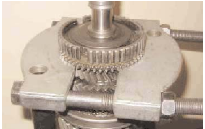
11. Invert the mainshaft. As the 5th /6th -gear synchroniser hub is not symmetrical identify its orientation. Using a press, or suitable puller, remove the 5th /6th -gear synchroniser hub, synchroniser ring and 5th speed gear assembly. Note: Care must be taken to ensure that damage to the teeth on the synchroniser flange does not occur. (On an over-drive transmission it may be necessary to engage the press/puller also over the gear).
