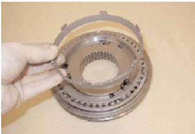
f) Remove the synchroniser friction ring.
