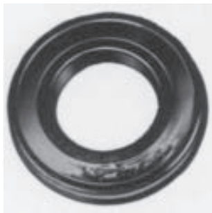
Bearing removed with punch, damaged shield.
