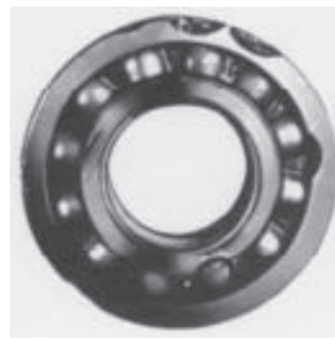
Bearing removed with chisel, damaged outer race.
