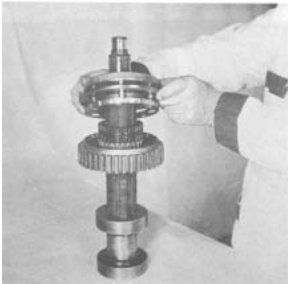
Figure 54 - Install 2nd & 3rd synchronizer assembly.
