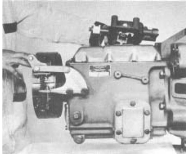
Figure 87 - Install remove control or shift control top, tighten bolts 20 to 25 ft. lbs. torque [27,2 - 33,8 N.m.].
