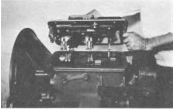
Figure 89 - Remove control cover assembly from transmission. Remove backup switch.
