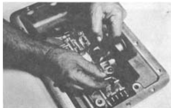
Figure 111 - Align one tapered interlock cross pin with hole in 1st & reverse shift rail. Position rail on poppet ball with rail in neutral position.
