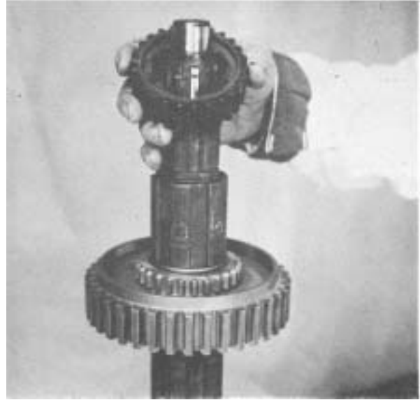
Figure 31 - Remove 2nd & 3rd shift hub sleeve.
