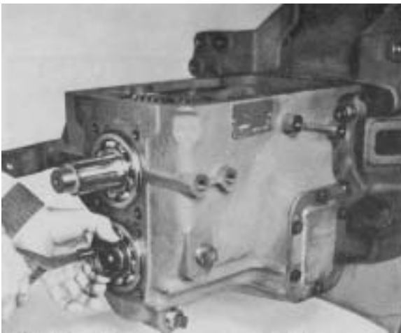
Figure 13 -Remove countershaft rear bearing cap.
