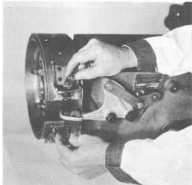
Figure 80 - Install brake release springs and cam lever shoe as shown.
