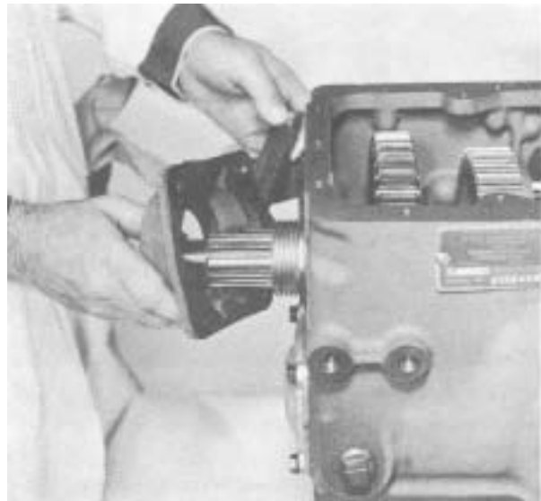
Figure 76 - Press a new oil seal in mainshaft rear bearing cap with lip of seal down. Coat a new gasket on both sides with a grade #2 multi-purpose grease. Position gasket on mainshaft rear bearing cap, use caution as not to cover oil return grooves in bearing cap. Install bearing cap with oil grooves lined up with oil holes in case. Tighten bolts 35 to 45 ft. lbs. torque [47,5 - 61,0 N,m].
