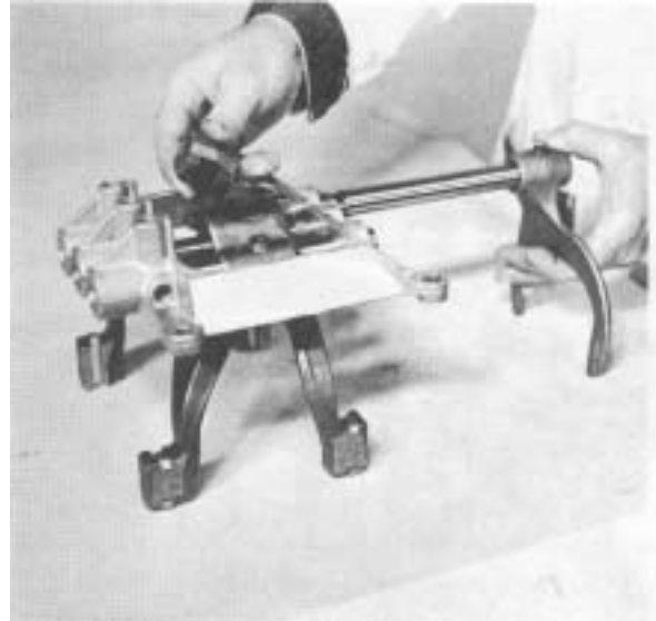
Figure 35 - Remove 1st & Reverse shift fork, rod and lug from shift rod support.
