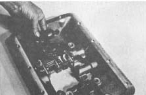
Figure 108 - Position 1st & reverse rocker arm on pivot pin as shown.
