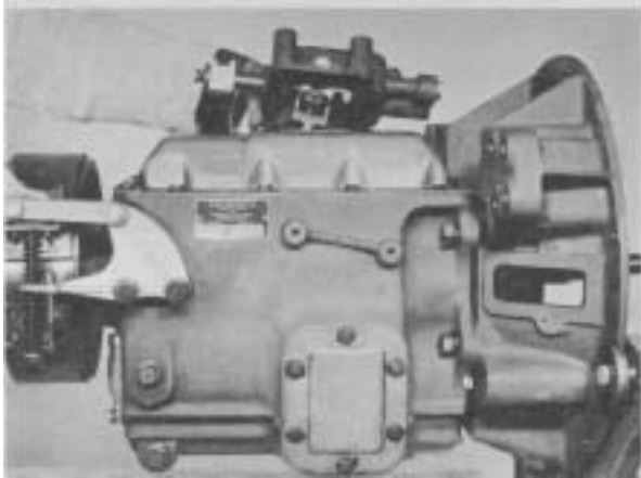
Figure 1-Remove control top or remote control assembly.
