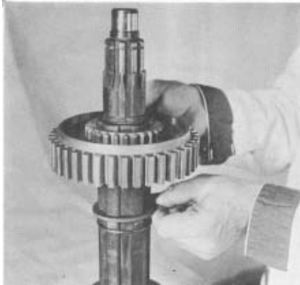
Figure 33 - Remove 2nd gear and locating washer.
