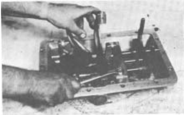
Figure 1 - Remove front and rear rail support capscrews.
