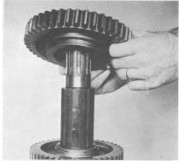
Figure 59 - Turn mainshaft assembly over and install 1st & reverse sliding gear with shift fork slot down.
