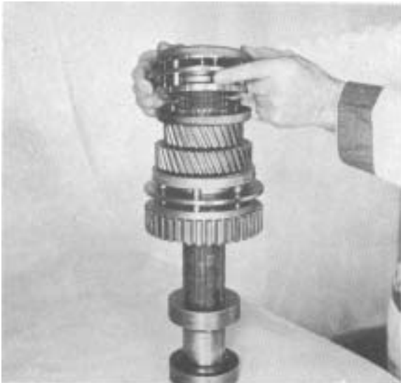
Figure 58 - Install 4th & 5th synchronizer on shift hub sleeve.
