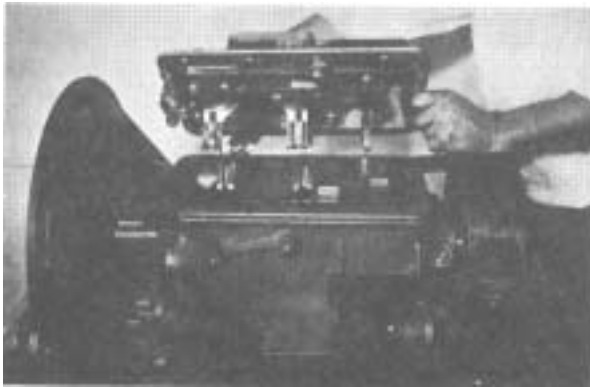
Figure 125 - With transmission in neutral, position control cover over gears aligning shift forks in shift cover with gear shift hubs. If control cover is in neutral and transmission is in neutral, transmission drive gear should turn without brake drum or output shaft turning.
