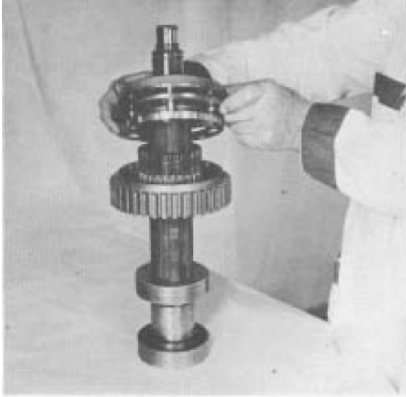
Figure 29 - Remove 2nd & 3rd synchronizer assembly.
