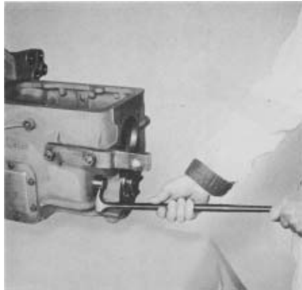
Figure 19 -Remove reverse idler shaft lockscrew and lock. Using a suitable puller remove reverse idler shaft.
