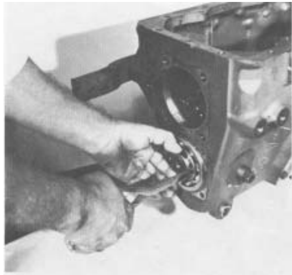
Figure 64 - Install countershaft rear bearing retainer ring.
