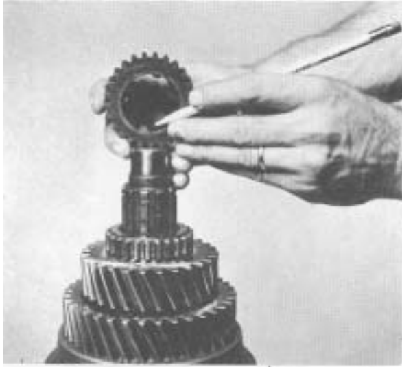
Figure 57 - Install 4th gear with clutching teeth up. Note chamfer on 4th & 5th shift hub sleeve. Chamfer must go down. Install bottom cup of 4th & 5th synchronizer on 4th speed gear clutching teeth before installing 4th & 5th shift hub sleeve. Install sleeve retainer ring.
