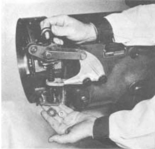
Figure 81 - With spacer link and cam lever in position, install adjusting bolt washer and nut.
