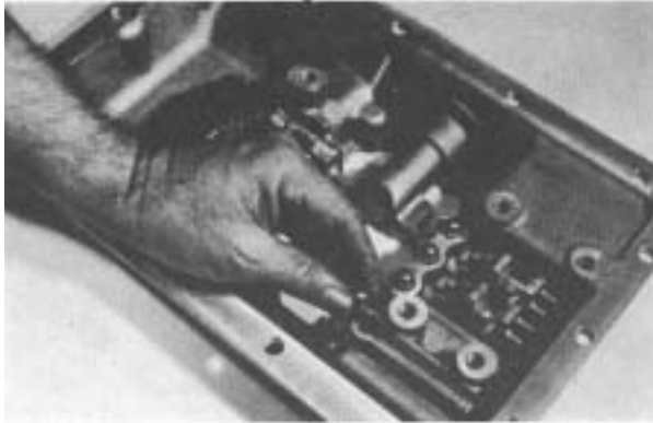
Figure 101 - Remove mesh lock poppet balls, quantity 4.
