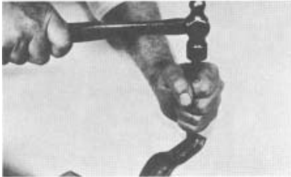
Figure - 106 - If fork bushings are worn, secure fork in a vise equipped with soft jaws and remove worn bushings with a drift. Install new bushings in fork. Turn fork over on anvil of vise and secure bushing in fork using a prick punch and upsetting bushing metal on outside of fork.
