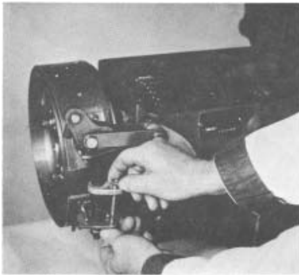
Figure 82 - Install band locating screw as shown with threaded end up; install nut.
