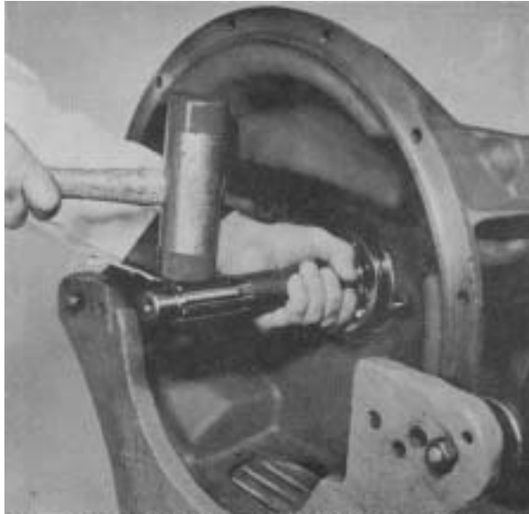
Figure 16 -Remove main drive gear. Use caution as not to drop mainshaft spigot bearing rollers in transmission case.
