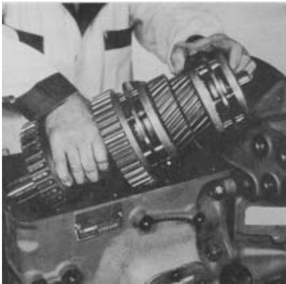
Figure 18 -Remove mainshaft assembly
