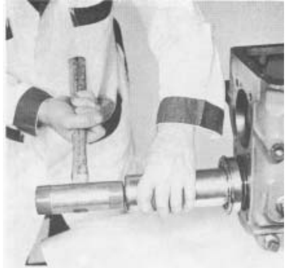
Figure 63 - Drive rear bearing on countershaft and rear bearing bore. NOTE: Countershaft drive gear must be supported on each side with a 1/4" flat bar to prevent damage to countershaft pilot bearing.
