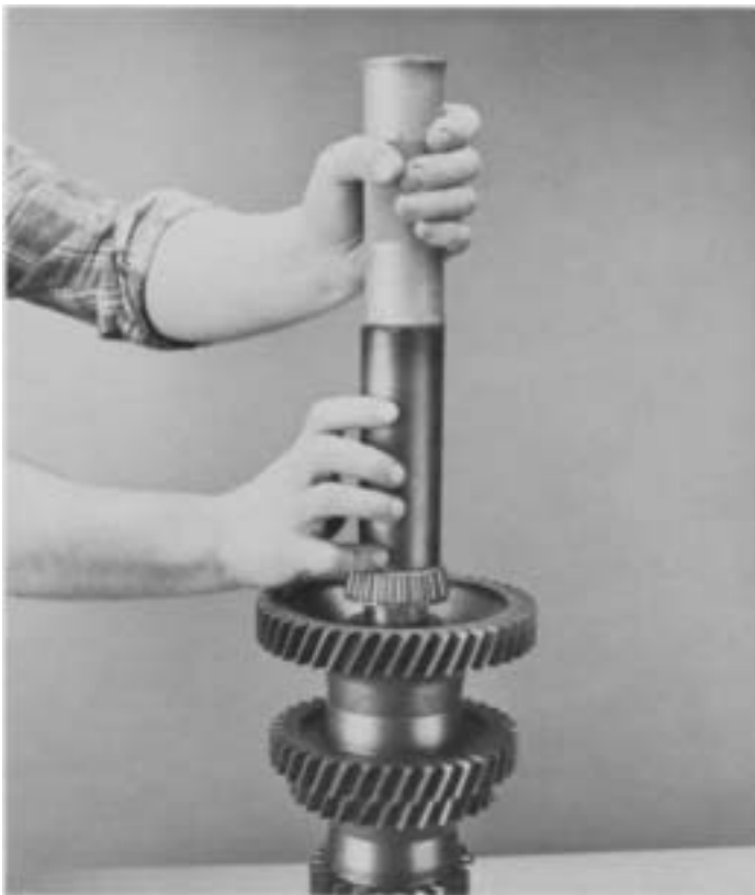
6. Install front countershaft bearing as shown.
