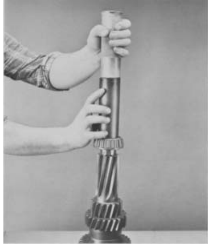
7. Install rear countershaft bearing as shown.
