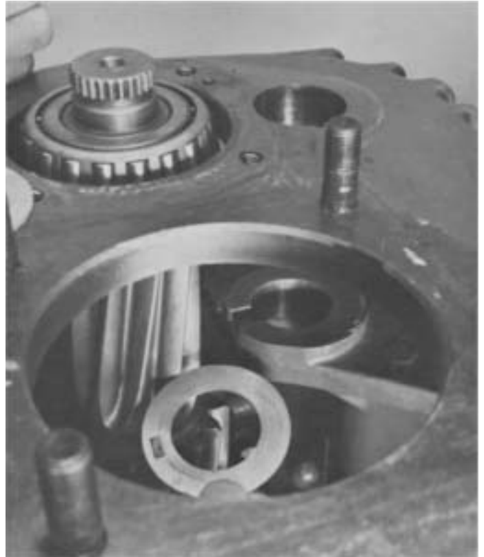
11. Use grease on reverse idler thrust washers to hold in place. Position tangs of washers in groove of housing.
