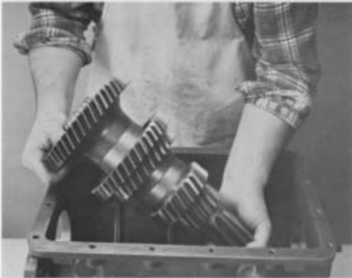
9. Carefully lower countershaft into case.
