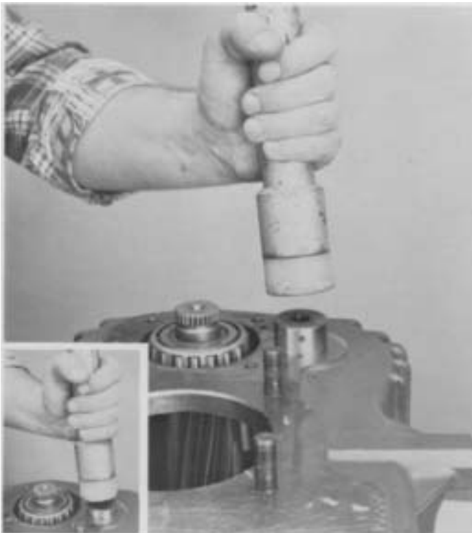
13. Insert idler shaft through case and idler gear bearings. Line up notch in shaft with notch in case, install lock ball, and drive shaft into position (inset).
