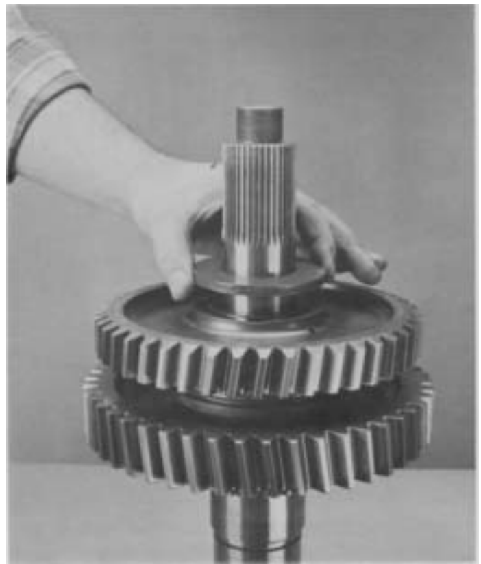
8. Install reverse gear washer. Washer can be installed either way.
