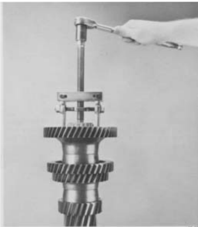
8. Position countershaft in vise, front of shaft facing up. Position puller jaws into notches behind front countershaft bearing and remove bearing.
