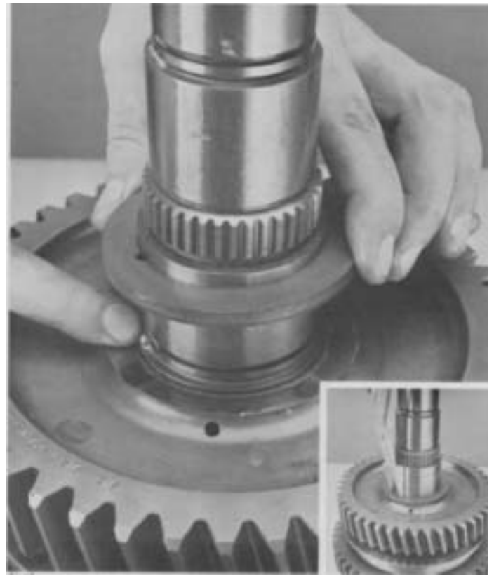
12. Remove snap ring (inset), thrust washer and locating ball.
