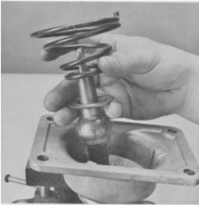
3. Remove tension spring, washer and gearshift lever from housing.
