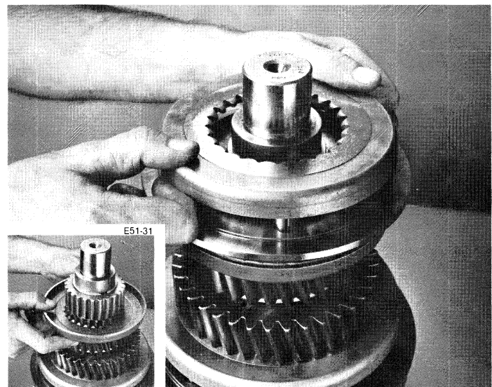
18. Install 5th gear synchronizer cup (inset). Lubricate friction surface with transmission lube and install 5th-6th synchronizer assembly and 6th gear synchronizer cup.
