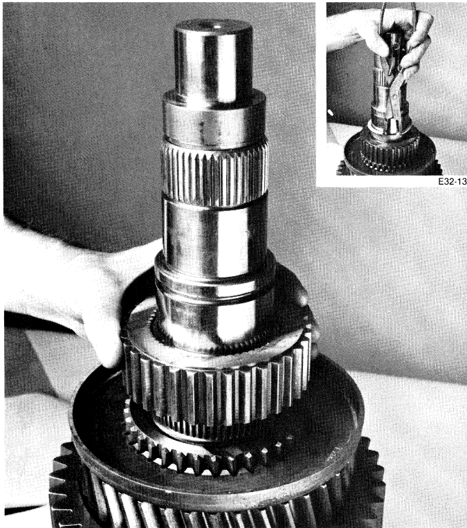
13. Remove snap ring from front of 3rd-4th clutch hub (inset). Remove clutch hub from main shaft.
