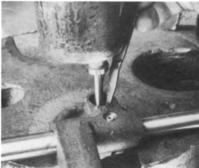
6. Place shift yoke in hand press. Depress retaining washer and spring and install the snap ring.
