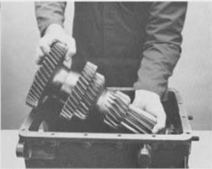
9. Carefully lower countershaft into case.
