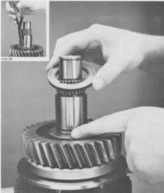
8. Remove snap ring (inset), thrust washer, and locating ball.
