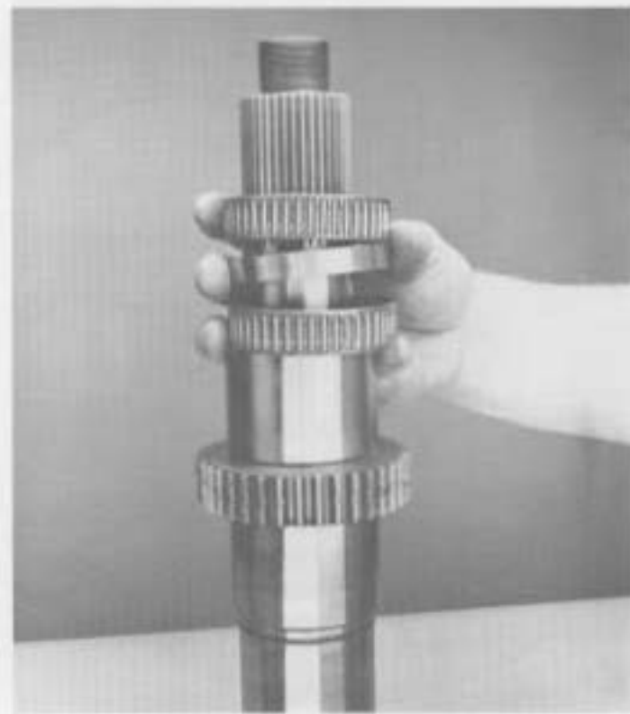
18. Remove reverse gear bearings and spacer from mainshaft.
