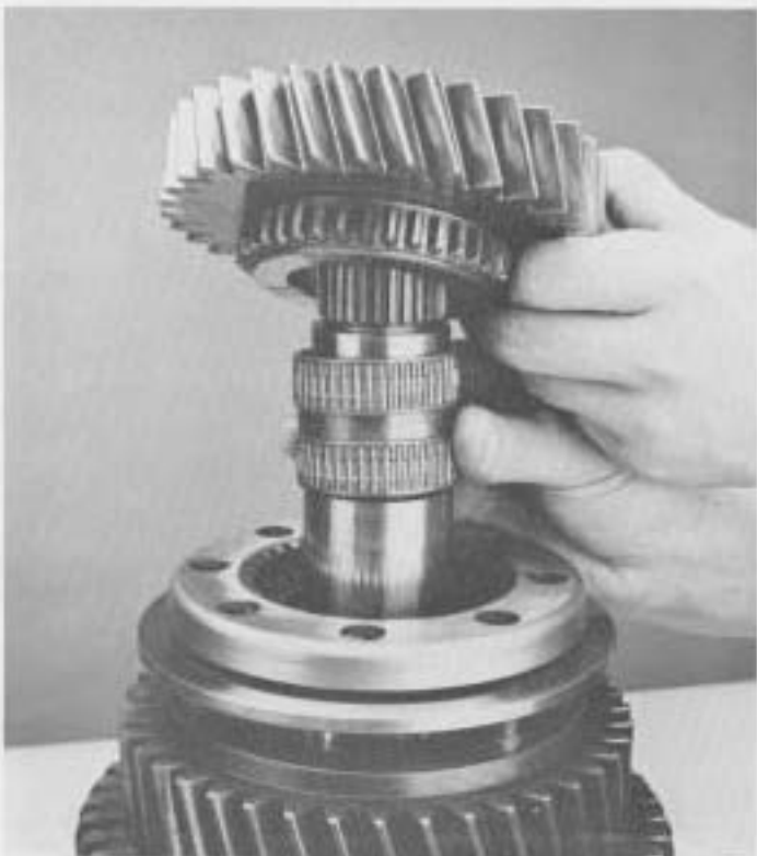
9. Remove 3rd gear, bearings and spacer from main shaft.
