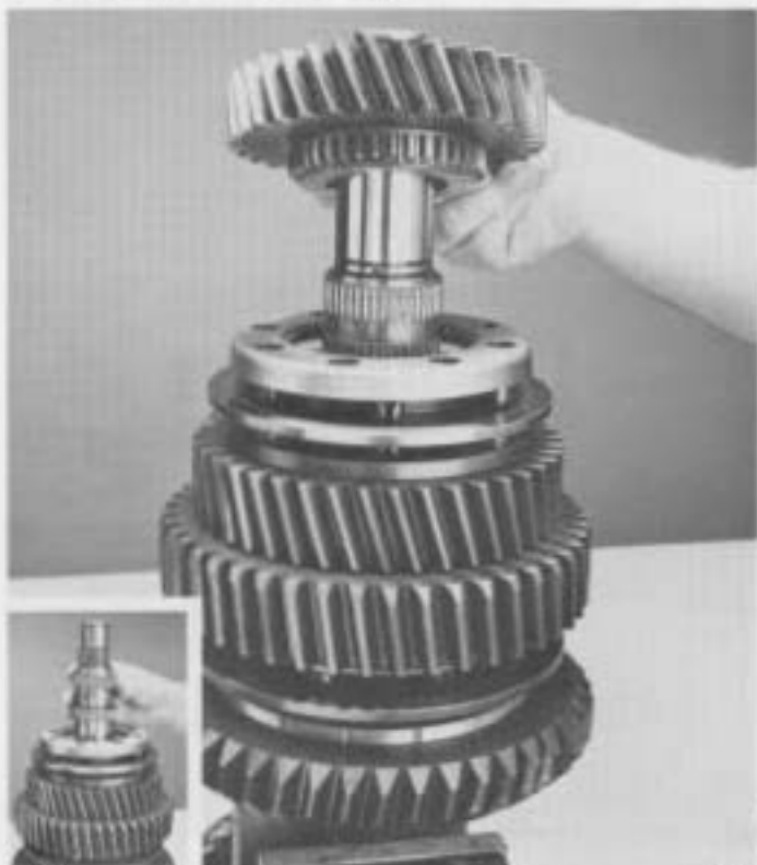
11. Lubricate and install 3rd gear bearings and spacer (inset). Install 3rd gear, clutching teeth facing down.
