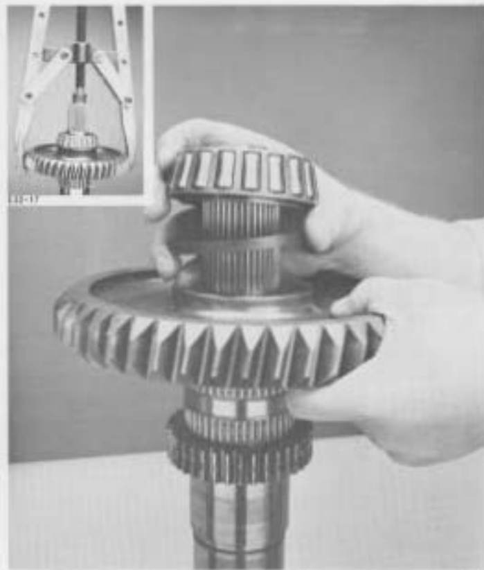
17. Using a puller (inset), remove reverse gear, washer, and rear bearing.
