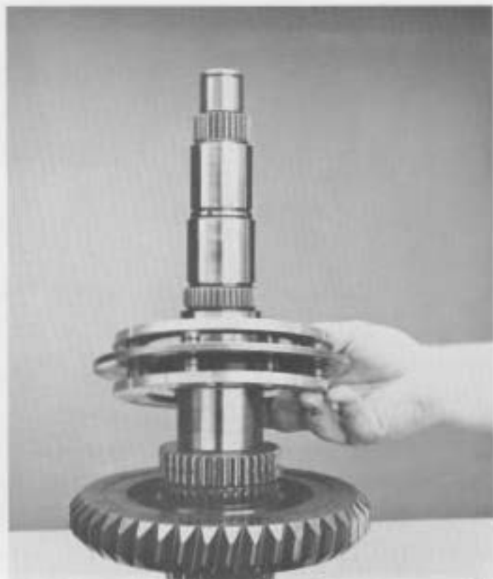
15. Remove 1st speed synchronizer.
