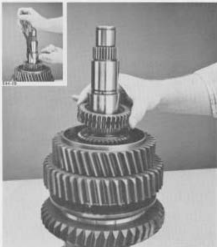
9. Install 2nd-3rd clutch hub with stepped face of hub facing up. Install snap ring in groove of mainshaft (inset).
