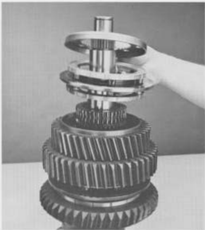
10. Lubricate friction surface with transmission lube and install 2nd-3rd speed synchronizer and 3rd speed synchronizer cup.
