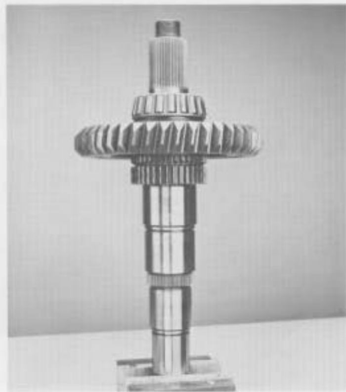
16. Reposition mainshaft in vise, rear of shaft facing up.
