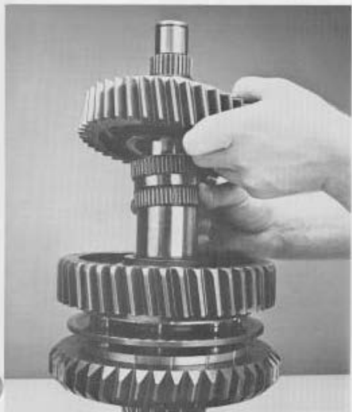
12. Remove 2nd gear, bearings, and spacer from mainshaft.
