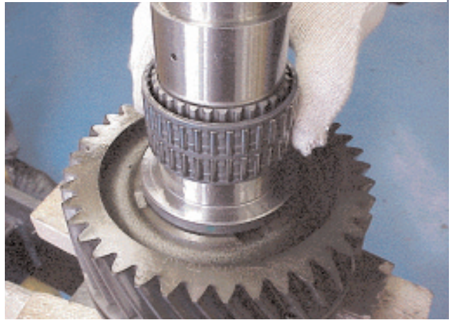
11. Remove the low gear needle roller bearing. Separate the low gear synchroniser hub, flange, ring and gear.
