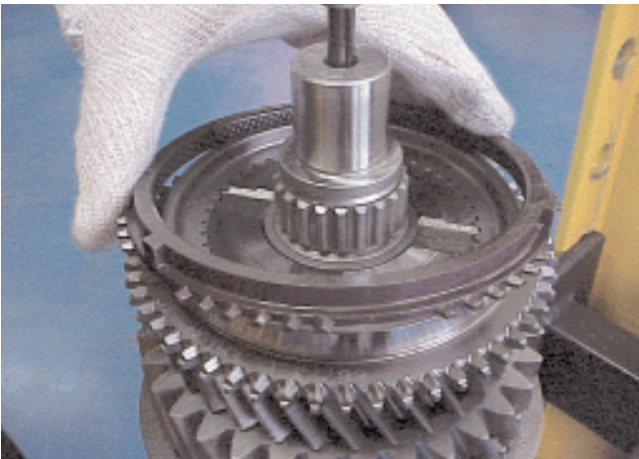
27. Lubricate the synchroniser ring with transmission oil. Fit the 3rd gear synchroniser flange and synchroniser ring.
