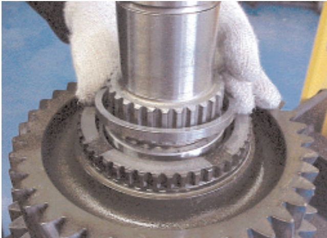
15. Install the bearing spacer ring into the gear and against the bearing.
