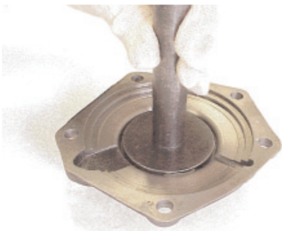
13. If removed, install a new oil seal into the input shaft bearing front cover using the special tool. Press the seal firmly down to the shoulder ensuring the seal is not damaged.
