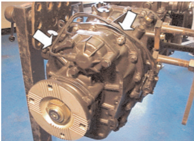
1. Using a hoist, mount the transmission onto the stand. Mark the hoses to ensure reassembly to the correct ports and disconnect the hoses from the transmission.
