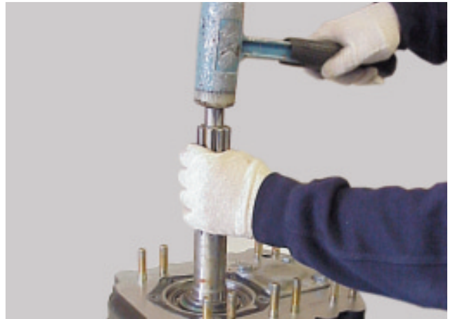
43. Use a soft faced mallet to drive the shaft through the case taking care not to allow the shaft to fall and become damaged.
