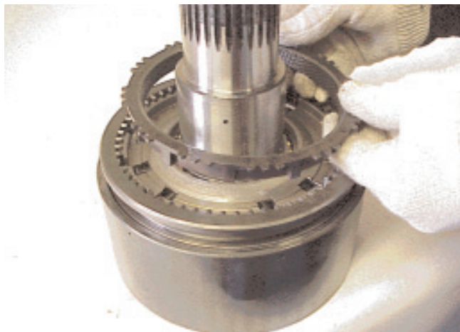
7. Lift off the synchroniser ring.
