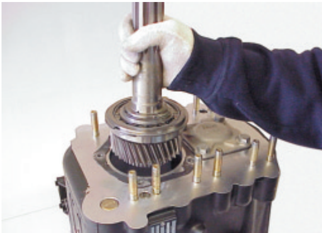
41. On direct drive models remove the input shaft and bearing assembly. Certain specifications have an O-ring seal/plate which must be removed before removing the input shaft cover.
