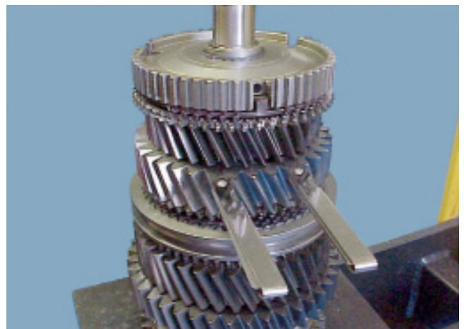
31. Check the gear end float using feeler gauges.
