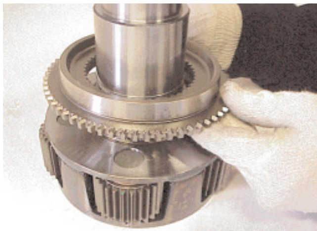
12. Remove the synchroniser flange.
