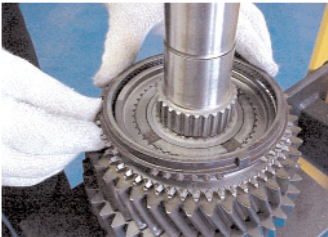
16. Install the 1st gear synchroniser flange to the gear. Lubricate and fit the synchroniser ring.
