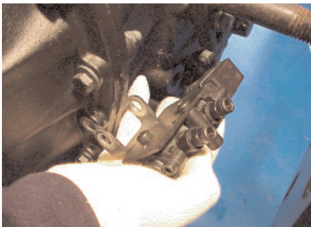
2. Remove the slave valve and mounting bracket (when mounted on the transmission). Protect the valve and hoses from dirt ingress.
