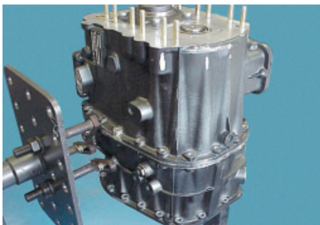
16. Locate the front case onto the intermediate case making sure the selector shaft enters the front bush and that the locating teeth on the input gear engage with the teeth on the synchroniser flange. Rotate the input shaft slightly to ensure engagement
