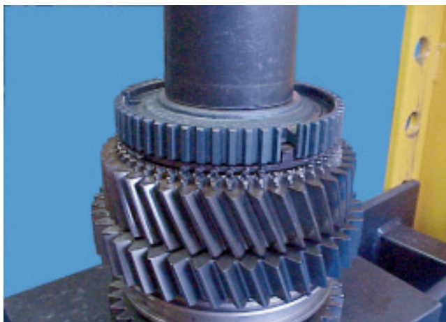
17. Support the mainshaft on the press. Place the heated 1st/2nd synchroniser hub over the splines on the shaft. Align the slots with the shoulders on the synchroniser ring and press the hub fully home. Check that the gear end float is within the tolerances stated in the chart.
