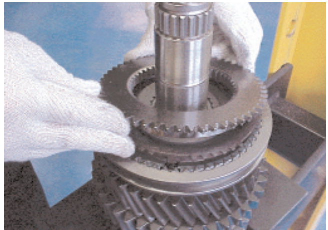
19. Lubricate the synchroniser ring with transmission oil. Place the 2nd gear synchroniser ring, ensuring that the shoulders of the synchroniser ring engage the slots of the synchroniser hub, onto the assembly. Place the synchroniser flange onto the assembly.
