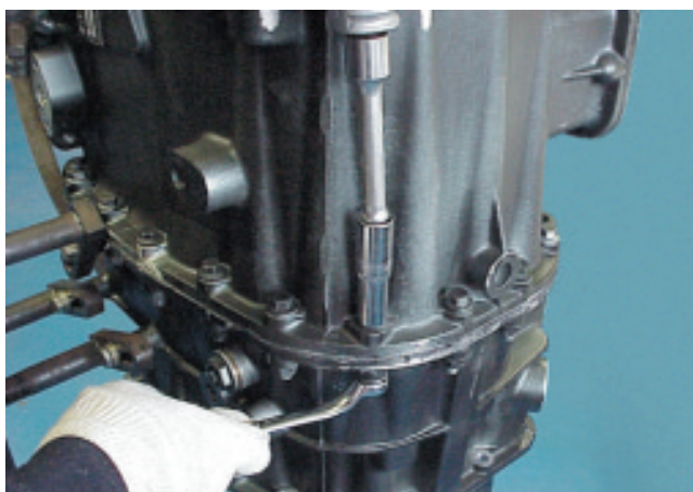
17. Install the flange capscrews, nuts and washers and tighten to the correct torque.
