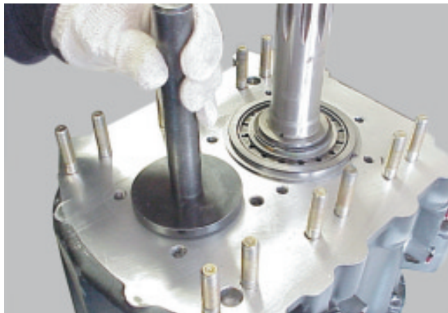
12. Install the layshaft front bearing cup into the front case assembly using tool E 109-6.
