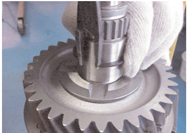
12. Invert the shaft and remove the 2nd gear bearing sleeve retaining snap ring.
