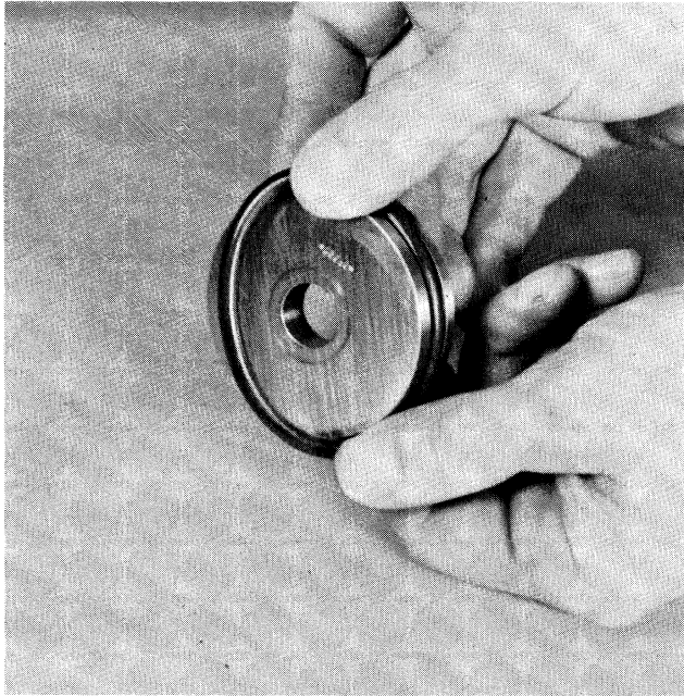
88. Installing O-ring on OD of piston.
