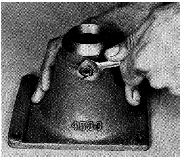
172. Installing lockwasher and nut to secure pivot pin.
