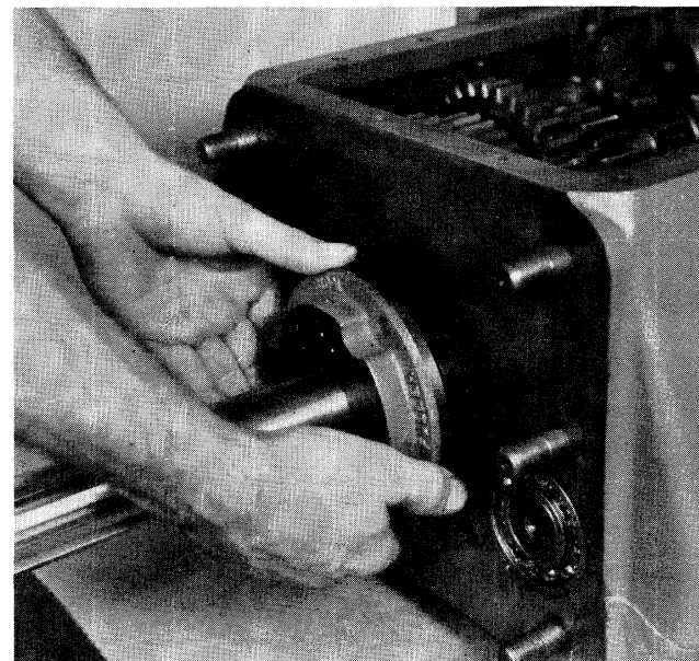
20. Removing the drive gear bearing cover.
