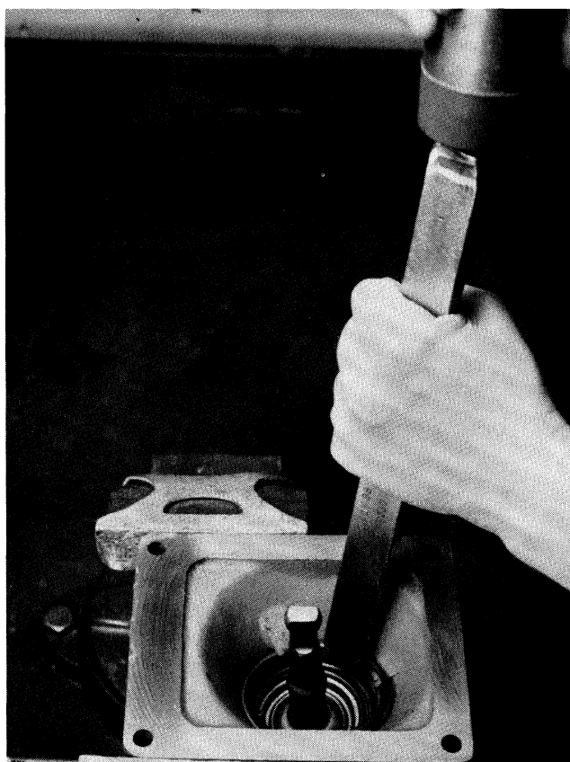
175. Installing the tension spring.
