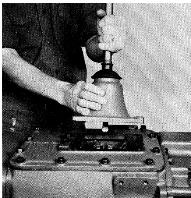
176. Installing the gear shift lever housing.
