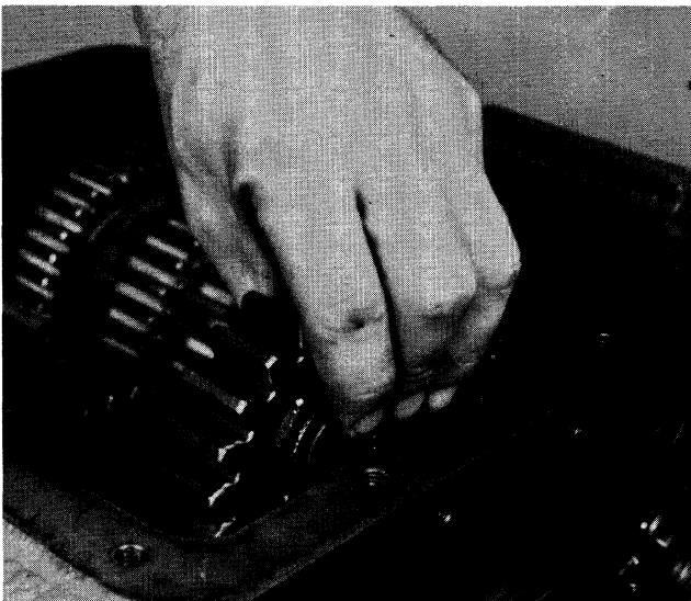
153. Placing reverse-idler gear into position in case.
