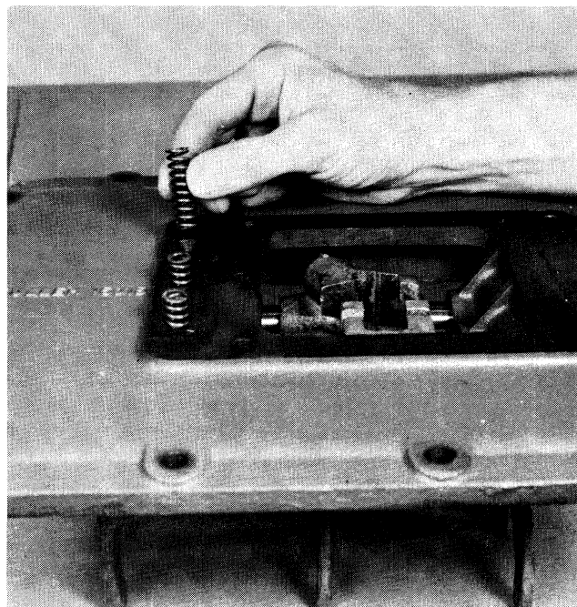
169. Installing tension springs in bores in top of housing.
