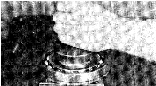
36. Driving auxiliary drive gear from bearing.
