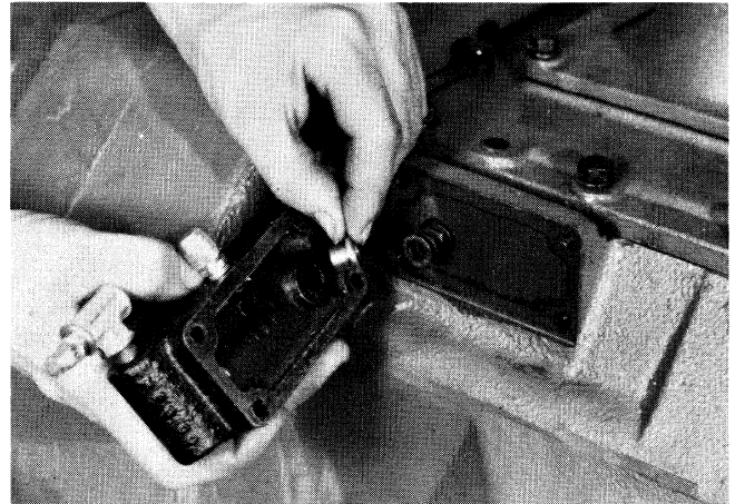
16. Remove the hat-type sleeve from the bore in the valve.
