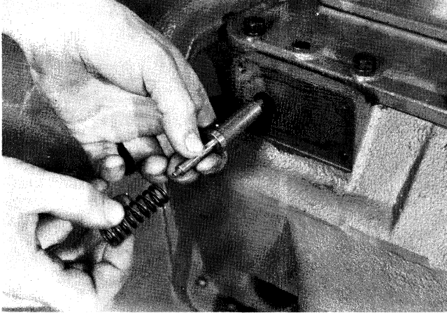
1. Install the actuating pin and spring in the bore in the case.
