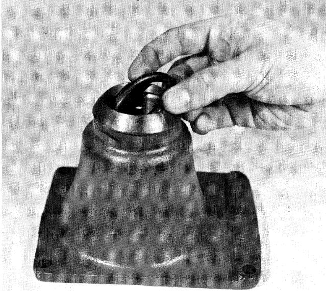
1. If so equipped, install the O-ring in groove in the housing.
