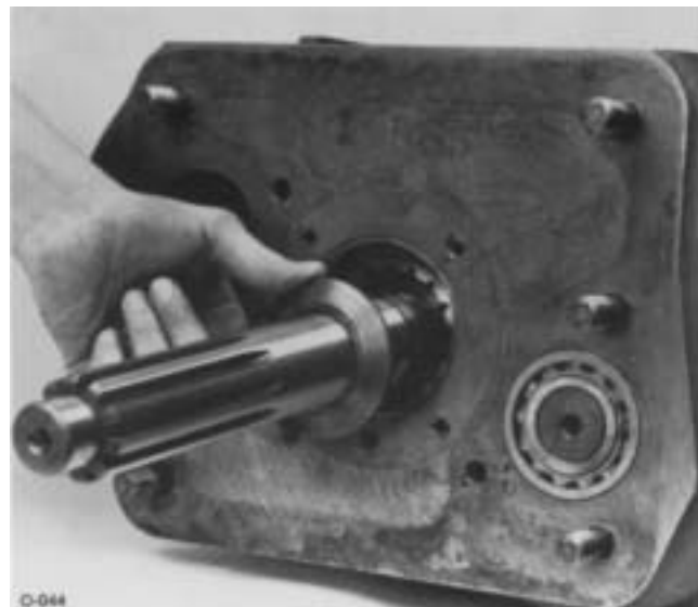
13. Install drive gear spacer on input shaft.
