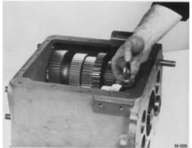
5. Remove the front idler washer from case
