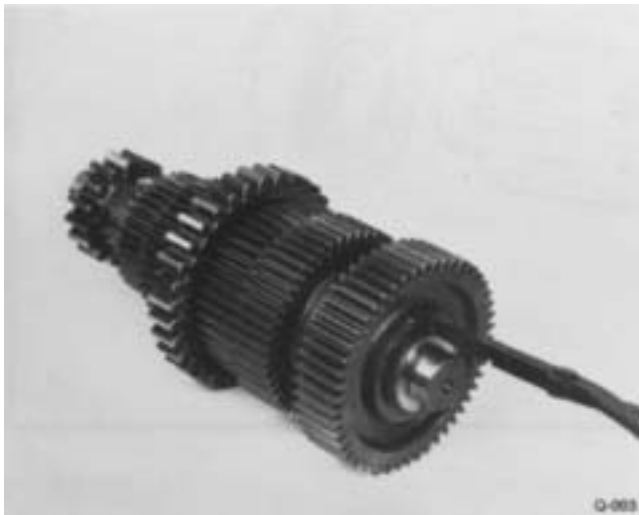
1. Remove snap ring from front of countershaft.
