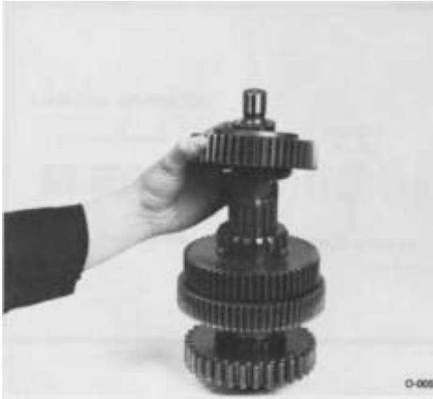
5. Remove the 3rd speed gear and washer.
