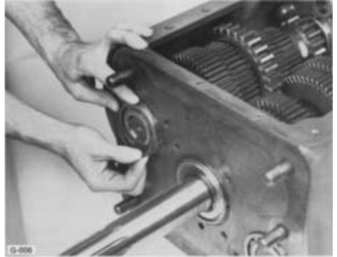
3. Install snap ring in the exposed bearing snap ring groove. (Use snap ring which was removed from rear bearing bore.)
