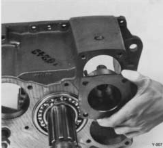
2. Remove cylinder from housing.
