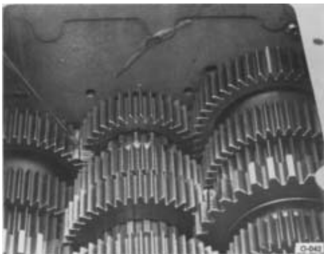
11. Mesh the marked timing tooth of left counter-shaft drive gear with the two marked timing teeth of the main drive gear.
