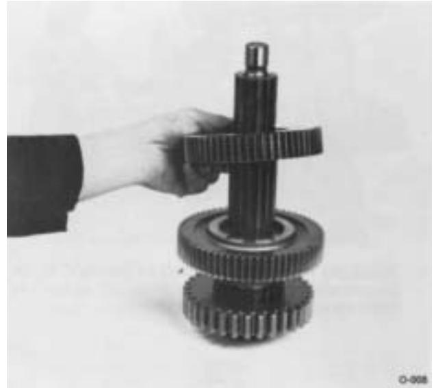
8. Remove the 2nd speed gear and washer.
