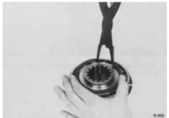
2. Install bearing retaining snap ring in groove of auxiliary drive gear shoulder.
