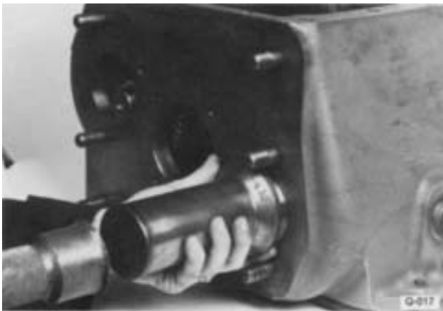
5. Install front bearing on countershaft and in case bore with flanged driver.
