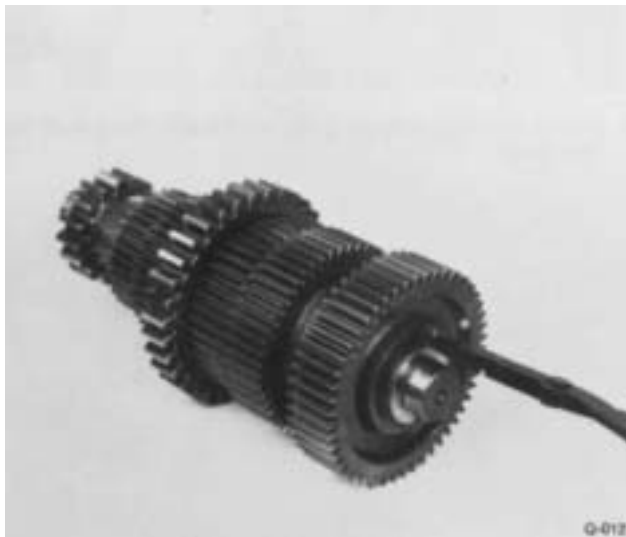
6. Install snap ring in groove at front of shaft.
