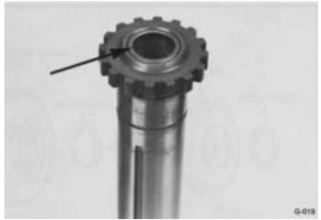
8. If necessary, remove bushing from pocket in clutch shaft.
