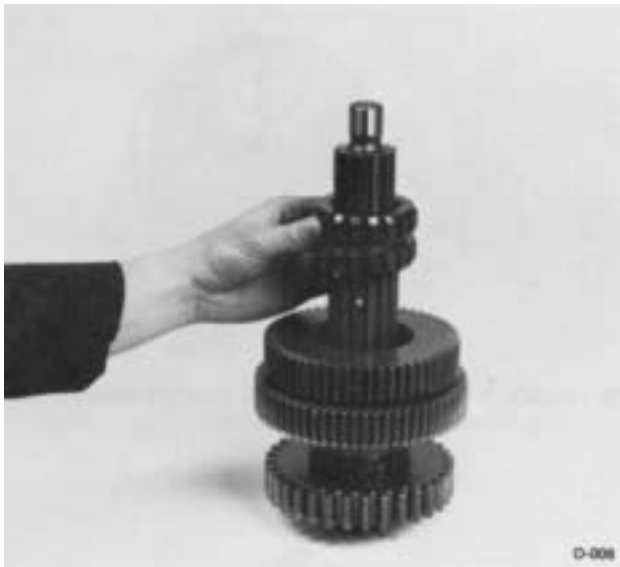
6. Remove the 2nd-3rd speed sliding clutch.
