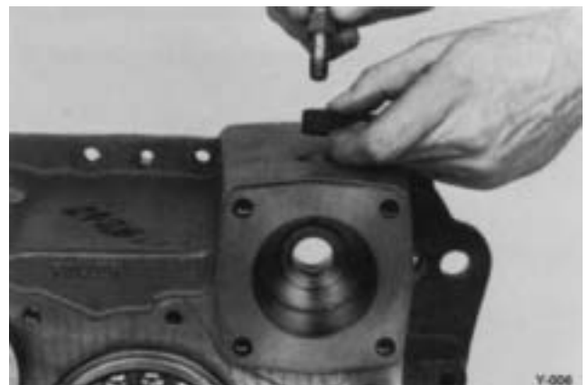
1. Important: Remove the dust seal, and air port extension from top of housing.
