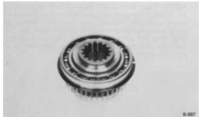
1. Press bearing on auxiliary drive gear, snap ring in groove towards gear.
