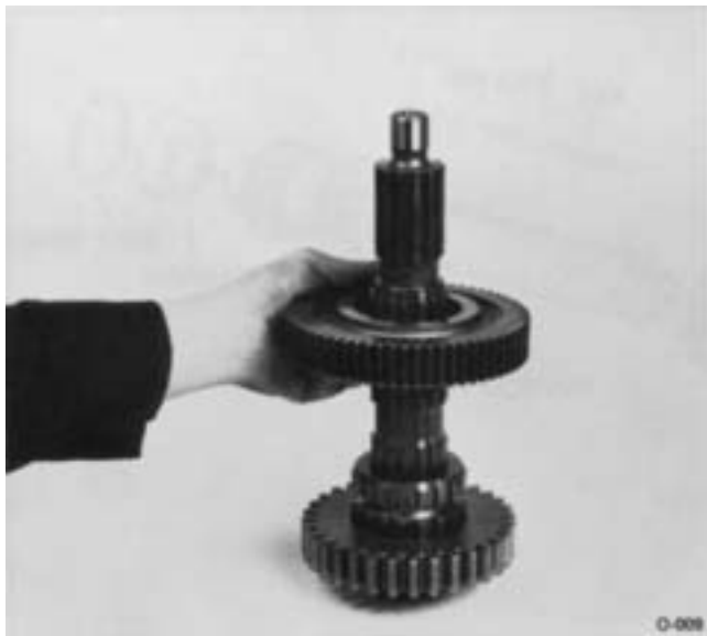
9. Remove the 1st speed gear and washer.
