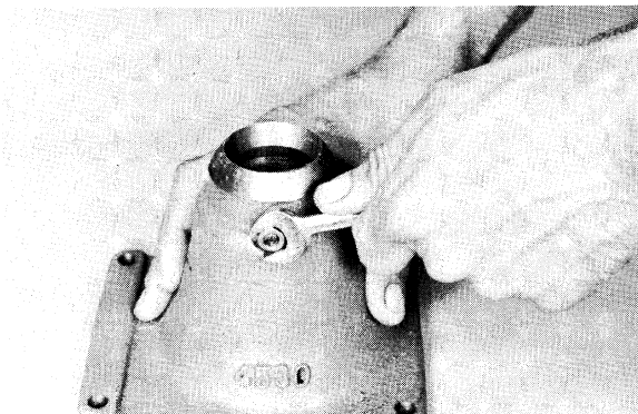
2. Install the pivot pin in the housing, threaded end out, and secure with the nut and lockwasher.
