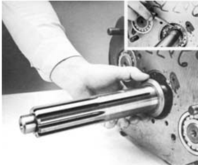
5. Remove drive gear spacer, and snap ring (inset.)
