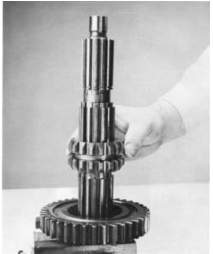
11. Remove Lo and reverse speed sliding clutch.
