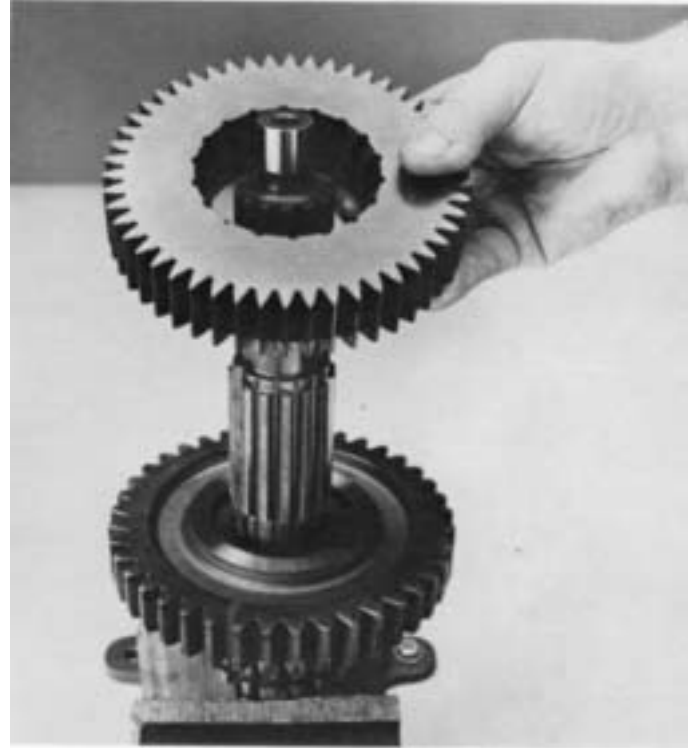
12. Install first speed gear on mainshaft, clutching teeth up.
