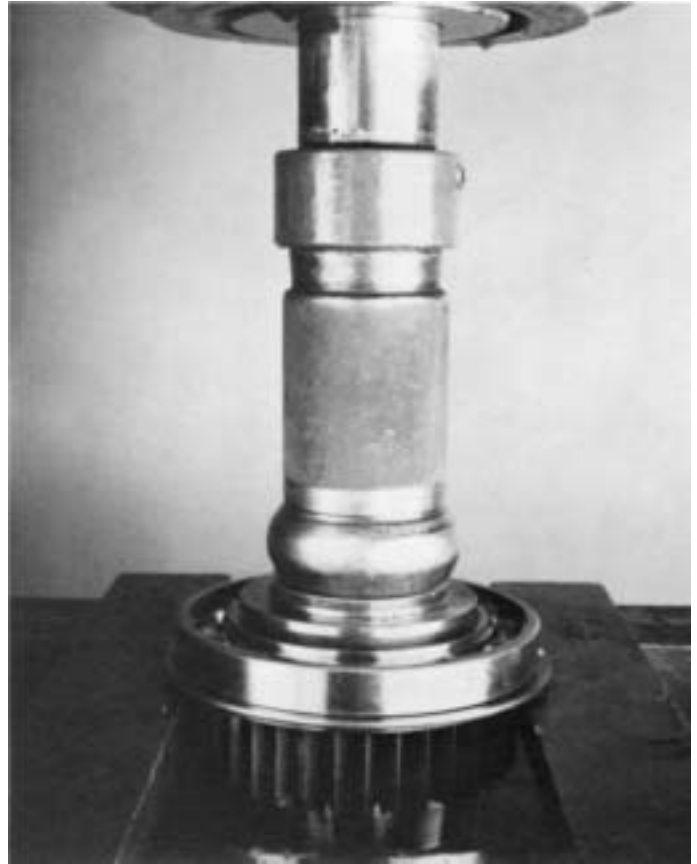
5. Press or use a driver to remove bearing from auxiliary drive gear.
