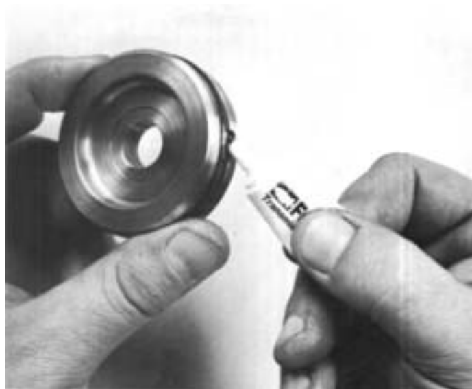
4. Install O-ring on O.D. of piston. Apply light coat of silicone lubricant to O-ring.
