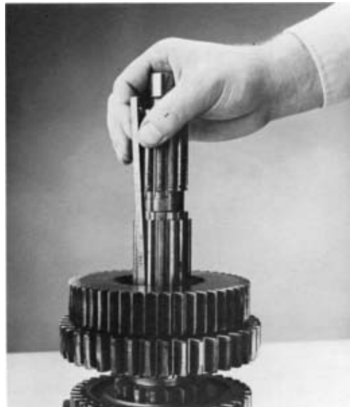
8. Remove the mainshaft key from keyway in mainshaft.
