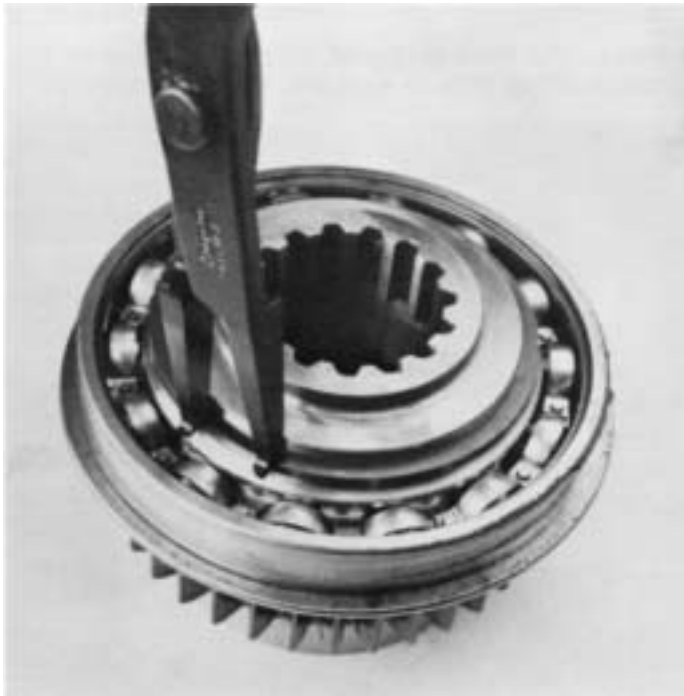
4. Remove snap ring from auxiliary drive gear.
