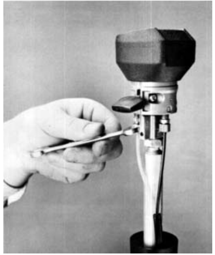
7. Connect the white air line to the "S" or Supply Port and the black air line to the "P" Port on the Roadranger valve. Tighten fittings securely.
