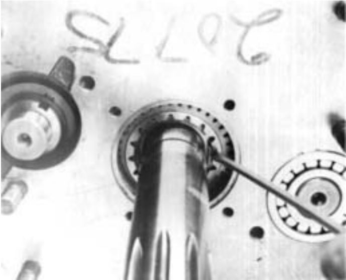
8. Install snap ring in snap ring groove inside drive gear.
