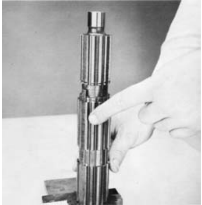
8. After proper reverse gear clearance has been set, remove the snap ring from rear of mainshaft, remove auxiliary drive gear and the reverse gear from mainshaft. The tolerance washer and key remain on the mainshaft. Reposition mainshaft in a vise as shown, pilot end up, so that the keyway is accessible.
