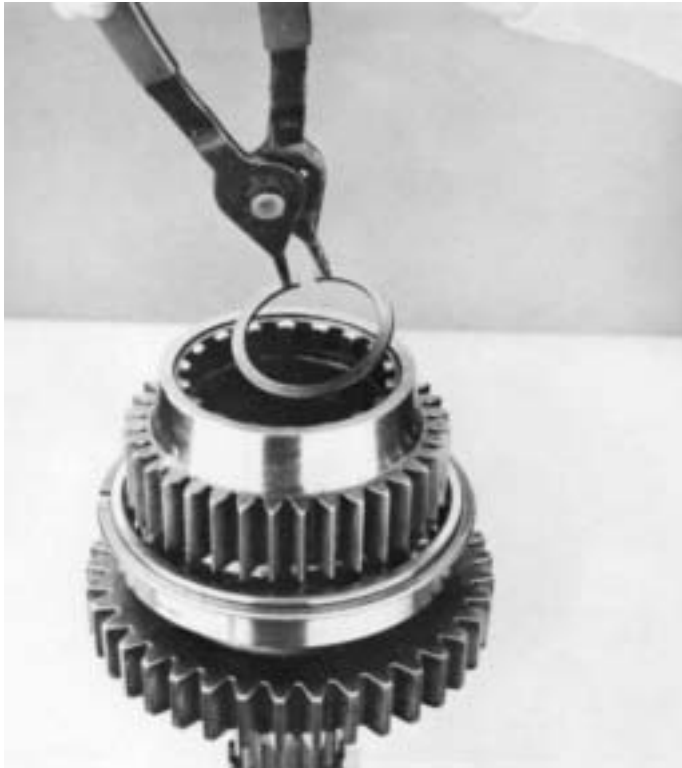
6. Install snap ring in groove at rear of mainshaft.
