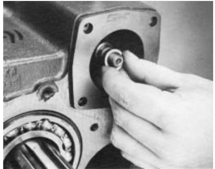
5. Remove the copper gasket from yoke bar.
