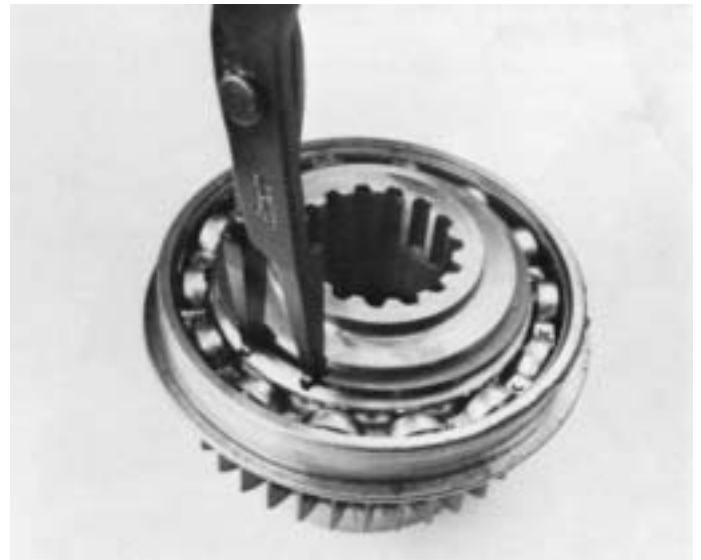
2. Install bearing retaining snap ring in groove of auxiliary drive gear shoulder.
