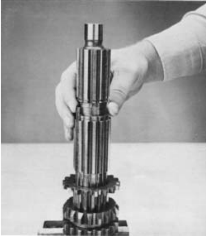
10. Remove mainshaft key from mainshaft. Install Lo speed gear tolerance washer on mainshaft Lo speed gear location and reinstall the mainshaft key to lock tolerance washer to shaft.
