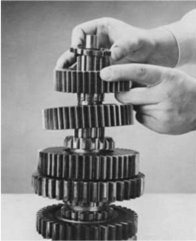
5. Remove 3rd speed gear and tolerance washer.
