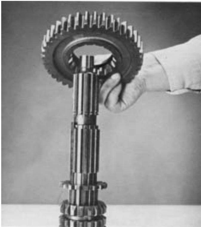
11. Install Lo speed gear on mainshaft, clutching teeth down, and engage with external splines of spacer.
