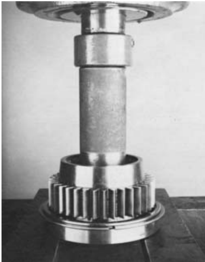
1. Press bearing on auxiliary drive gear.
