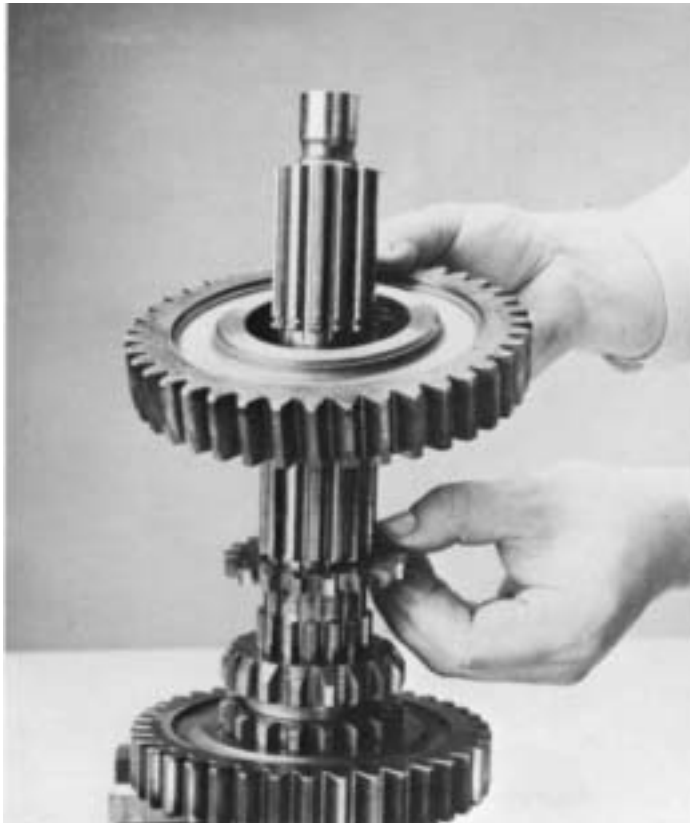
10. Remove Lo speed gear and tolerance washer.
