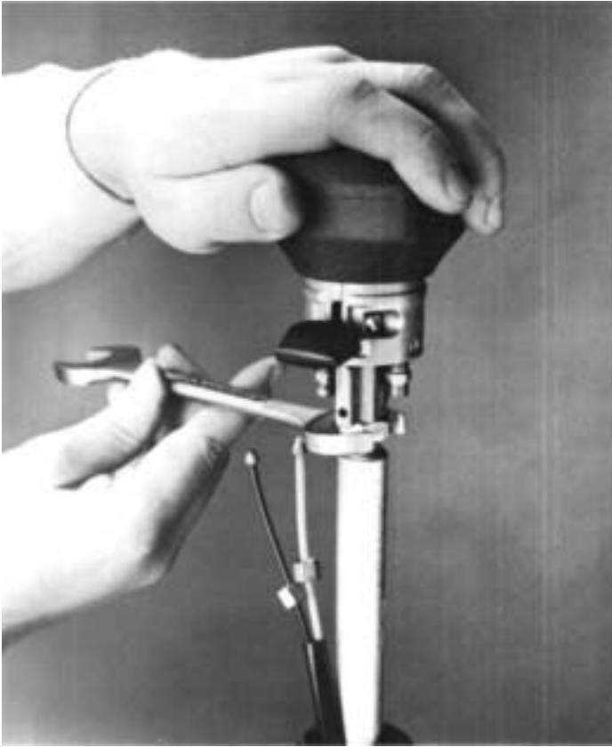
5. Position air lines, valve cover and jam nut on shift lever. Thread the Roadranger valve on shift lever and secure by tightening jam nut against valve.
