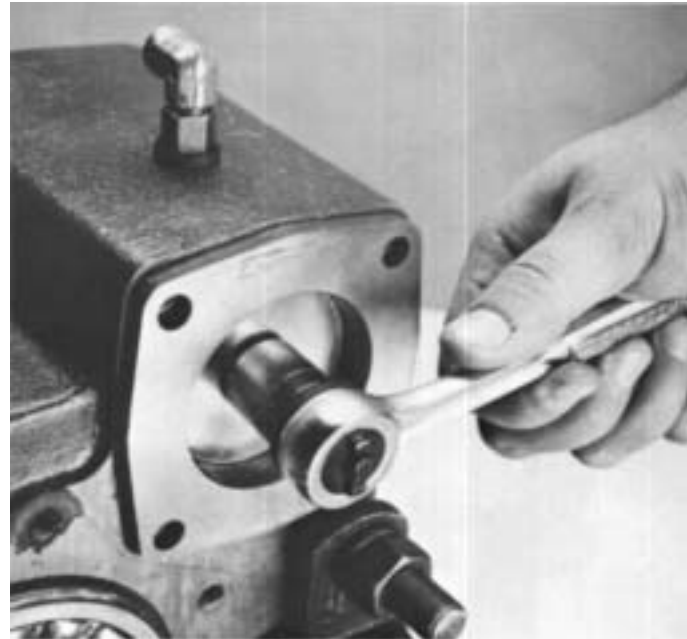
6. Install lockwasher and nut on yoke bar to secure piston. Tighten nut to recommended torque.
