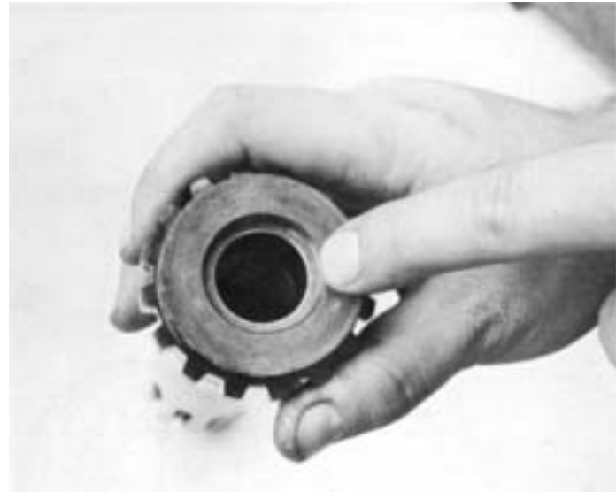
7. Check the bushing in pocket of input shaft, replace if worn.
