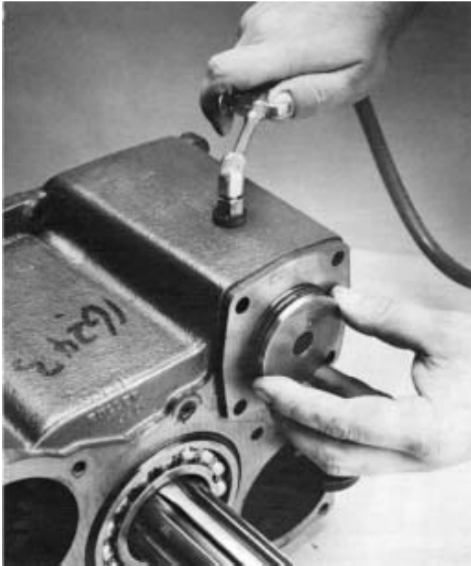
3. Use air to remove piston.
