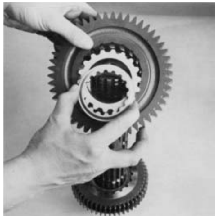
14. Lift 2nd speed gear from rear of mainshaft to remove limit washer, spacer, and gear. If necessary remove snap ring from I.D. of gear.
