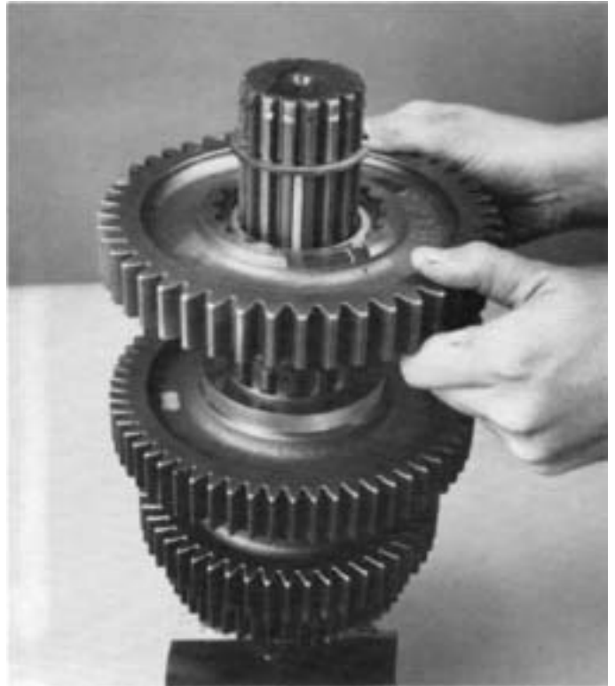
22. Install reverse gear on mainshaft, clutching teeth down and engaged with external splines of spacer.
