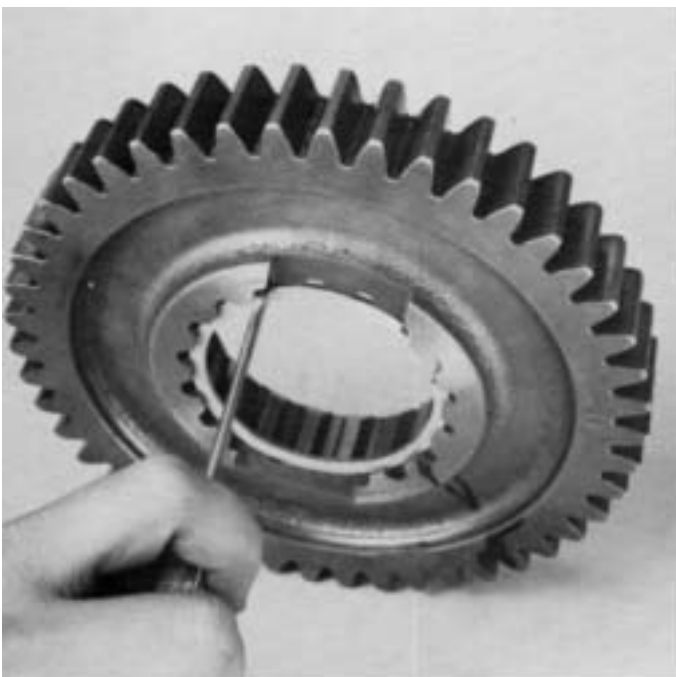
21. Install snap ring in hub of reverse gear ONLY TO CHECK AXIAL CLEARANCE (END-PLAY) LIMITS.
