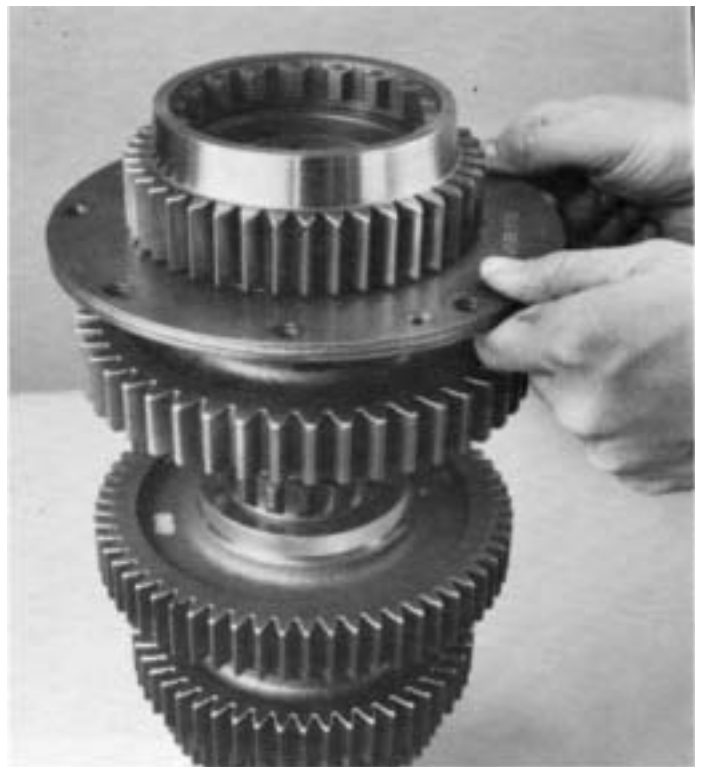
23. Install the auxiliary drive gear assembly in its proper position on rear of mainshaft.
