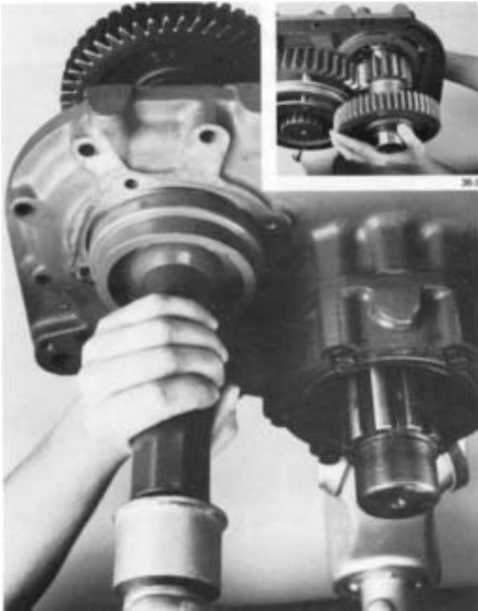
4. Install snap ring in groove at rear of each countershaft.
