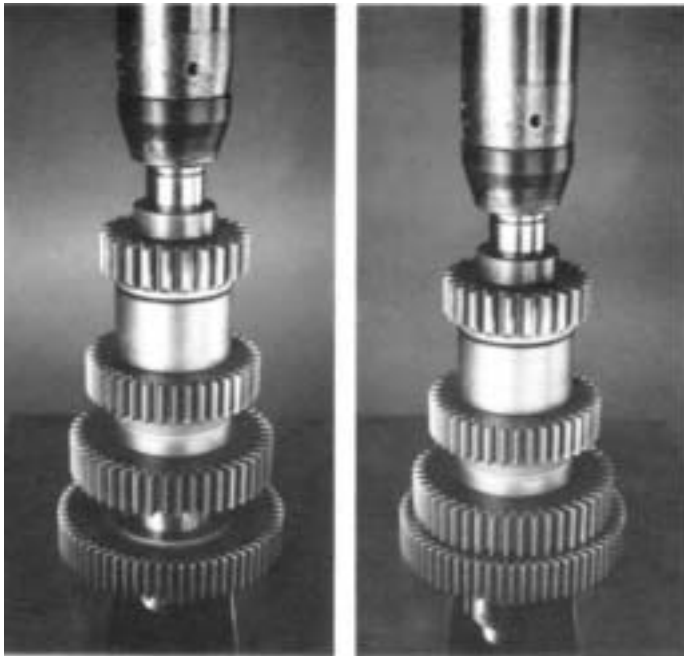
4. Press 3rd speed gear on countershaft, long hub of gear to front of shaft.
