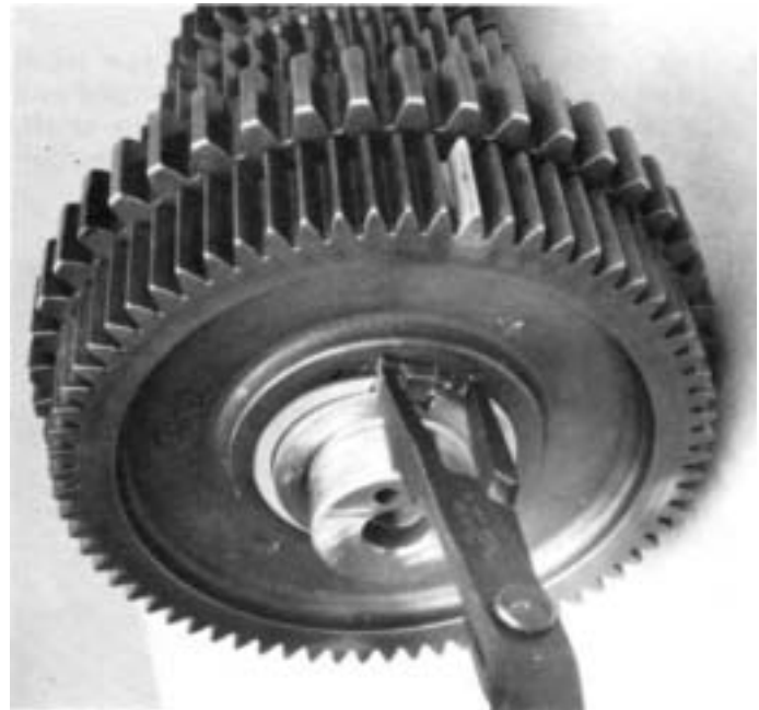
7. Install drive gear retaining snap ring in groove on front of each countershaft.
