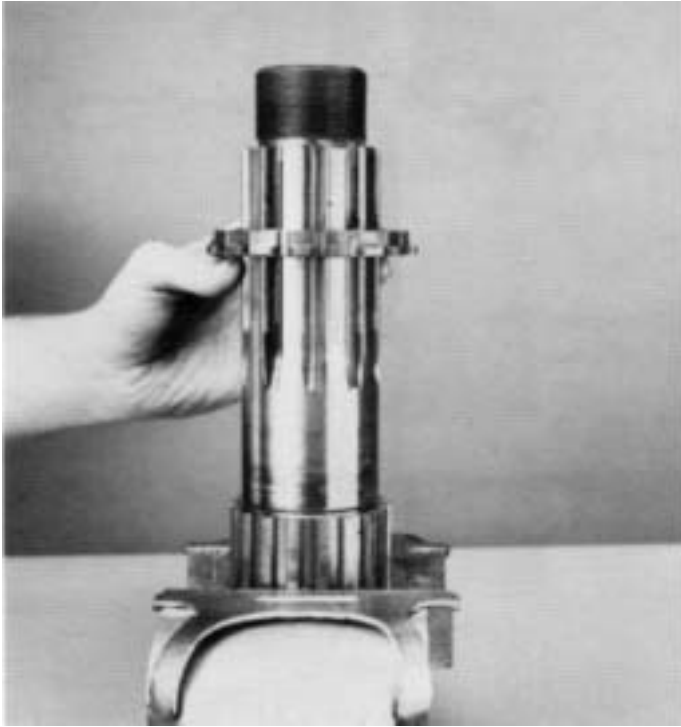
5. Remove splined spacer from output shaft.
