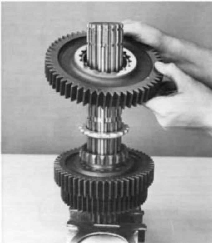
13. Install 1st speed gear on mainshaft, clutching teeth down and engaged with external splines of spacer.
