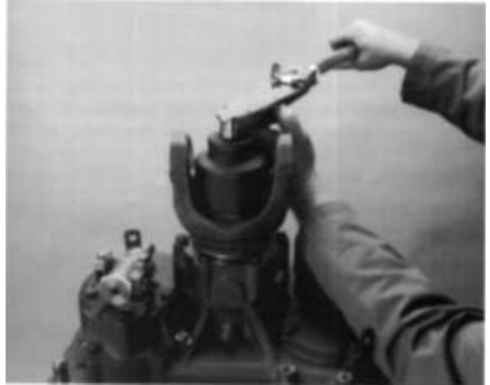
4. Complete installation process by torquing the output shaft nut to recommended torque.
