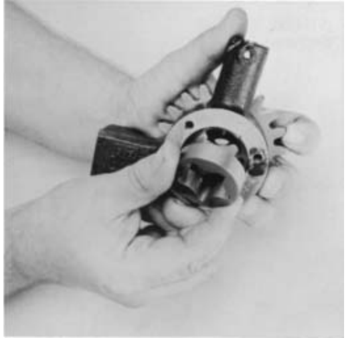
5. Remove outer oil pump element from pump.
