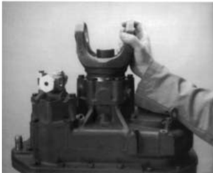
2. Place output yoke or flange onto the output shaft.
