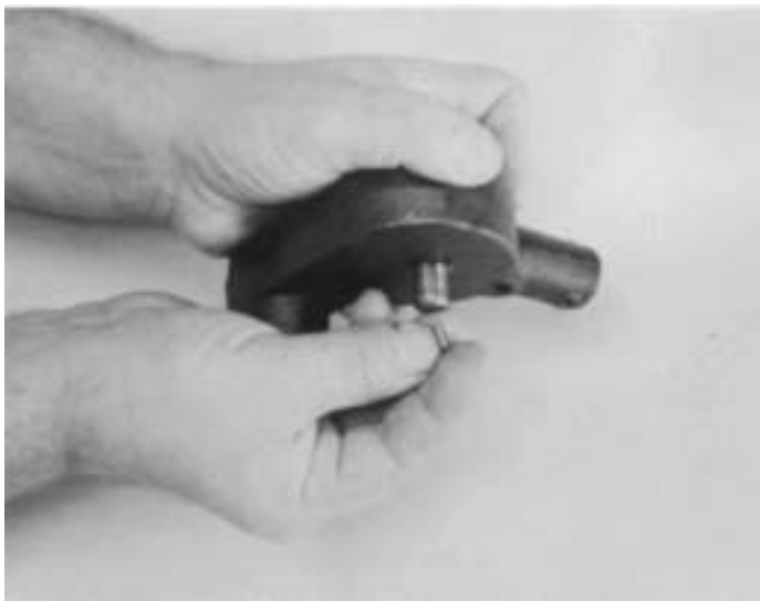
8. Remove key from drive shaft keyway.
