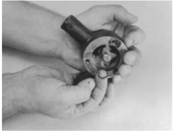
9. Remove element retaining snap ring from drive shaft.
