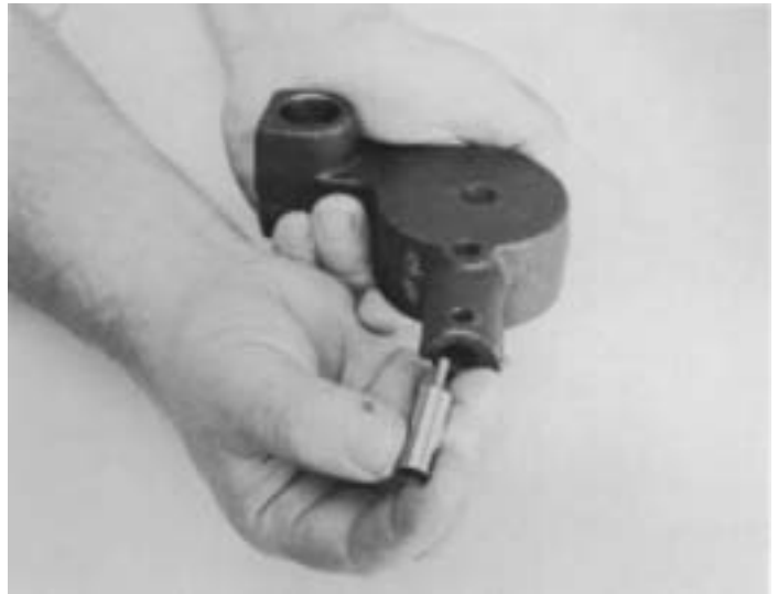
14. Remove relief valve from housing bore.
