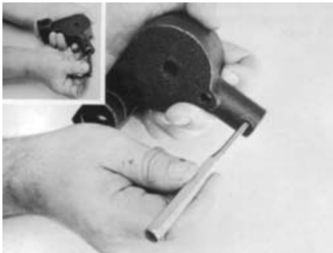
13. Remove relief valve roll pin from pump housing, relief valve spring can now be removed from relief valve housing bore (inset).
