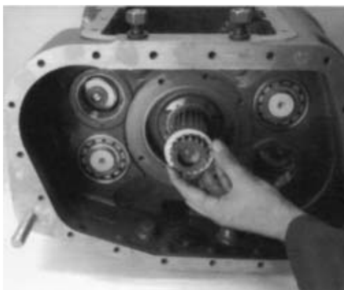
6. Remove the spline d washer from the mainshaft also remove the front auxiliary drive gear retaining snap ring from the mainshaft.
