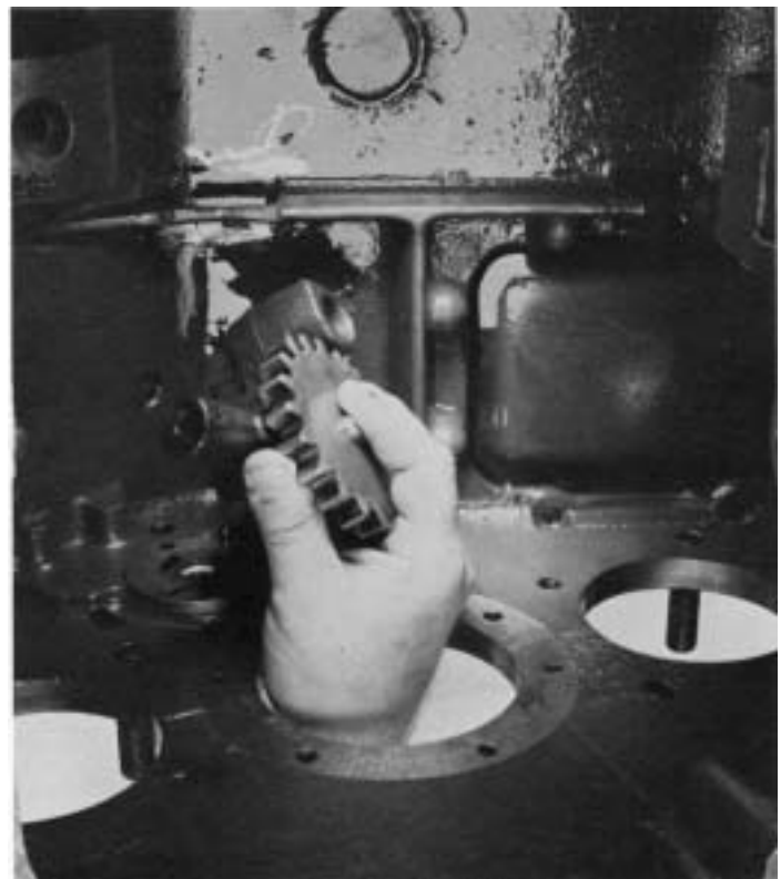
12. Install integral oil pump assembly in case aligning front face of oil pump with retainer and alignment pin.
