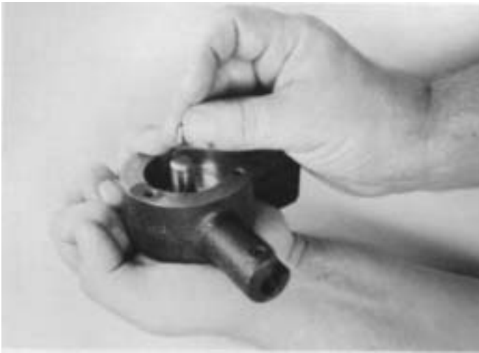
11. Remove two keys from drive shaft keyways.
