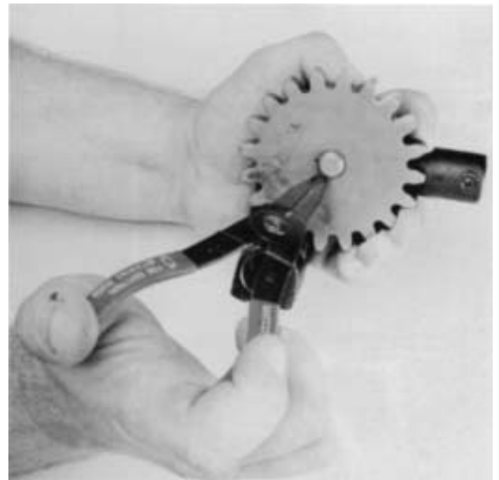
6. Remove drive gear retaining snap ring from drive shaft.
