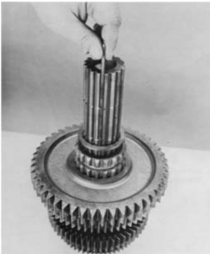
4. From mainshaft rear, pull the key from mainshaft key way.
