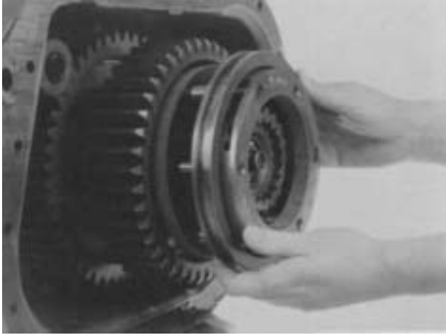
1. Slide the synchronizer from the mainshaft.
