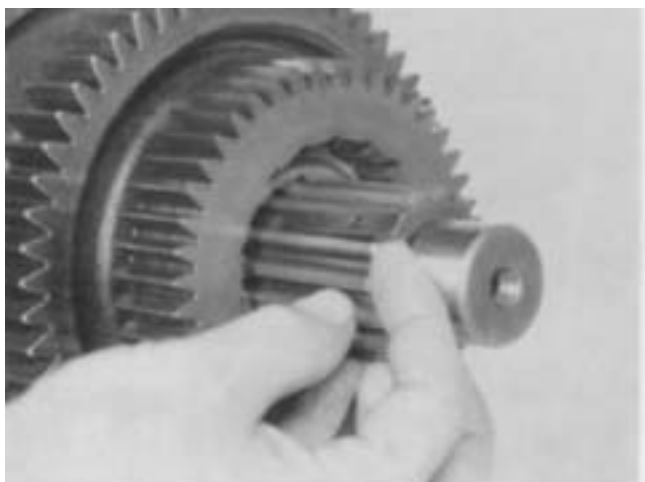
2. Lift the short key out of the groove in the mainshaft.
