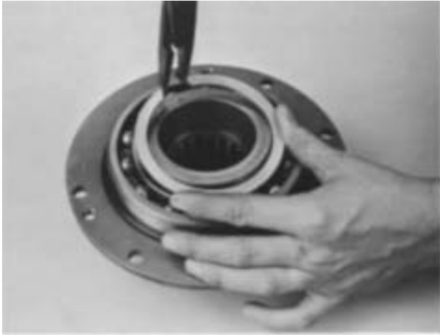
4. Remove the snap ring from hub of auxiliary drive gear.
