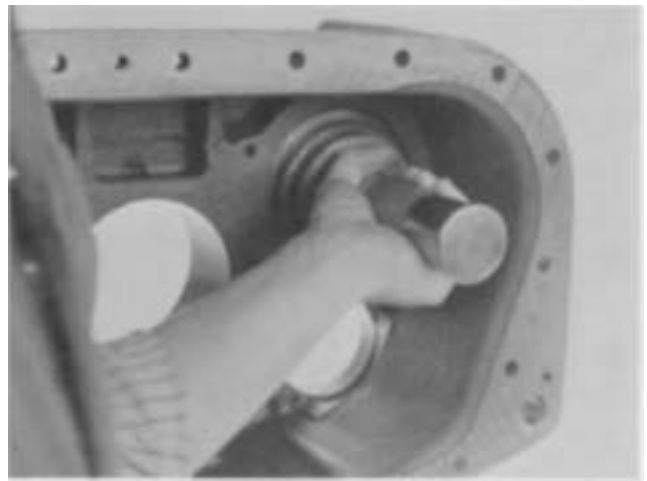
10. Drive out the two countershaft bearings.
