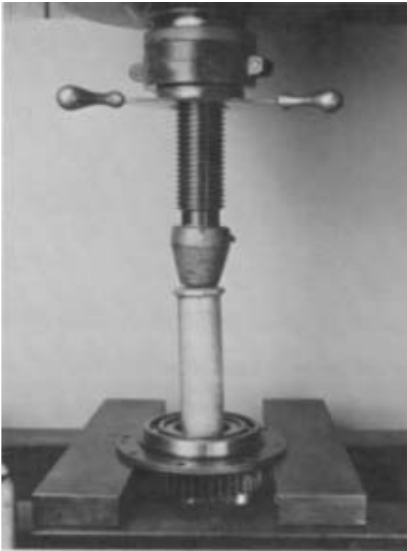
5. Using the rear face of retainer ring as a base, press the drive gear through bearing.
