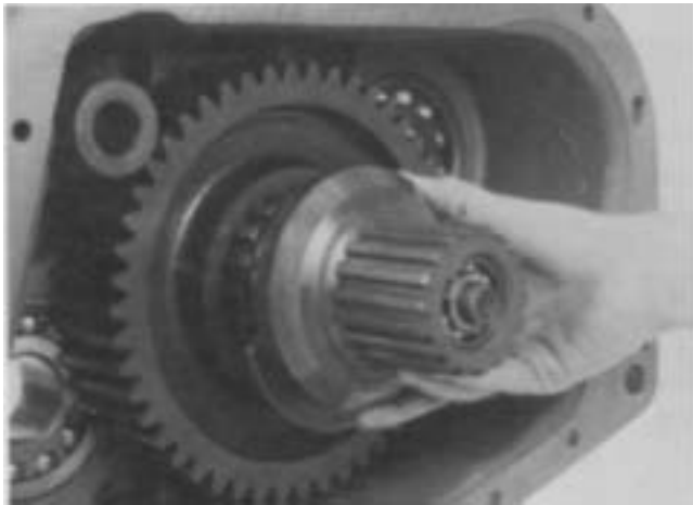
5. Slide the coupler off mainshaft.
