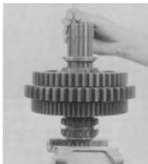
4. Clamp the mainshaft in a vise with brass or soft jaws and withdraw the long key.
