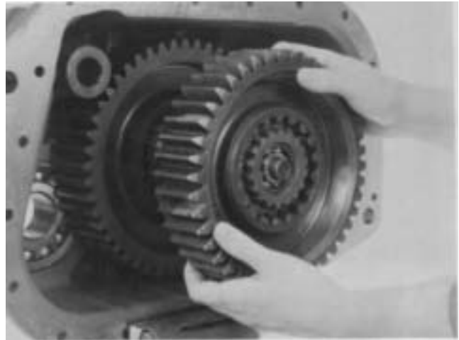
6. Install low range gear on mainshaft with machined surface facing machined surface on coupler.
