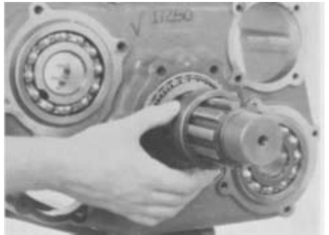
5. Slide speedspacer (or gear, depending on model) off output shaft.
