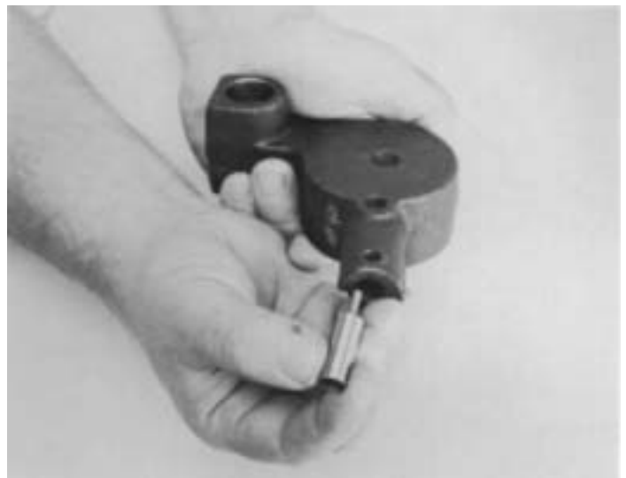
14. Remove relief valve from housing bore.
