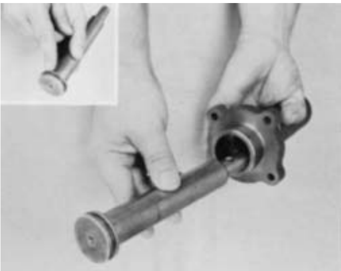
4. Pull the yoke bar from cylinder housing. If necessary, remove the O-ring from piston O.D. (inset).
