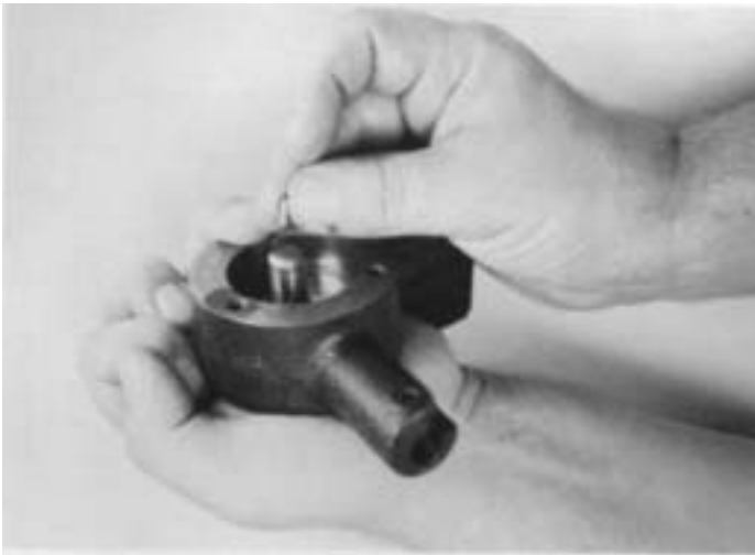
11. Remove two keys from drive shaft keyways.
