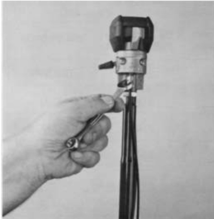
9. Connect the red air line to the "S" or Supply Port and the black air line to the "P" Port on the Roadranger valve. Tighten fittings securely.
