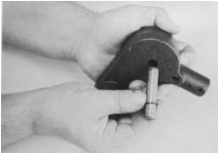
12. Remove the drive shaft from integral oil pump housing. If necessary, remove rear drive gear retention snap ring from drive shaft.
