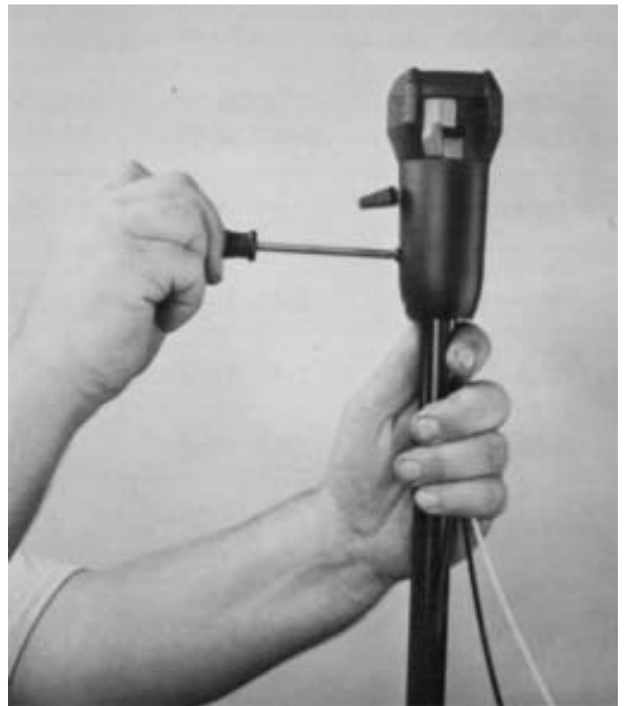
11. Position valve cover on Roadranger valve and secure by tightening the two mounting screws in cover,
