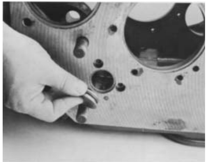
15. If necessary front case plug can be removed from case by driving the plug through front of case. Remove O-ring from O.D. of plug if necessary.
