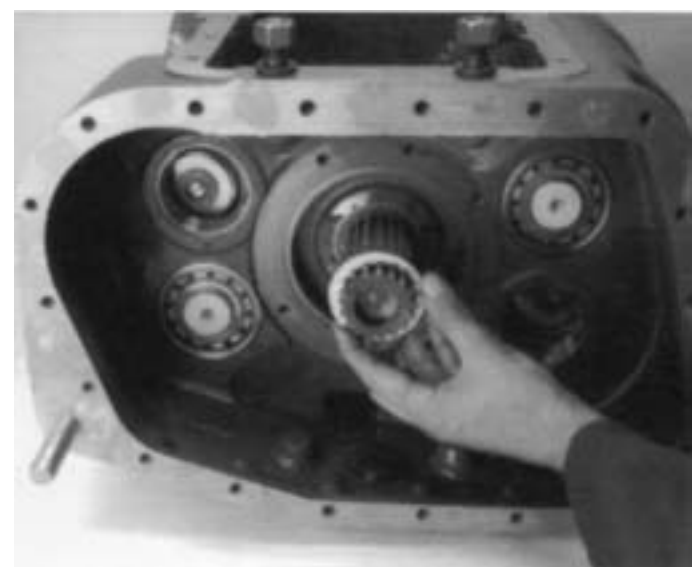
6. Remove the spline d washer from the mainshaft also remove the front auxiliary drive gear retaining snap ring from the mainshaft.
