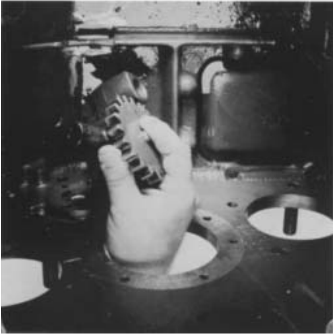
3. Remove the integral oil pump from case.
