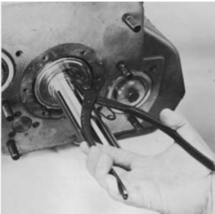
8. Install bearing retainer snap ring.
