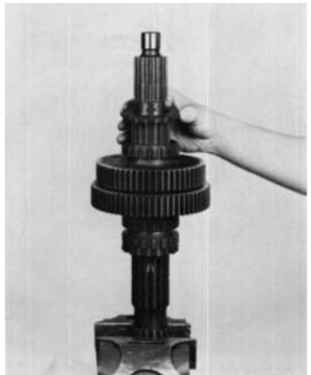
13. Lift the key and remove the 3rd speed gear splined washer.
