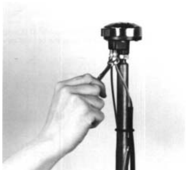
8. Disconnect the three 1/8" O.D. air lines at the selector valve.
