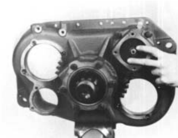
6. Install the piston on the shifting shaft, flat side of the piston facing out.
