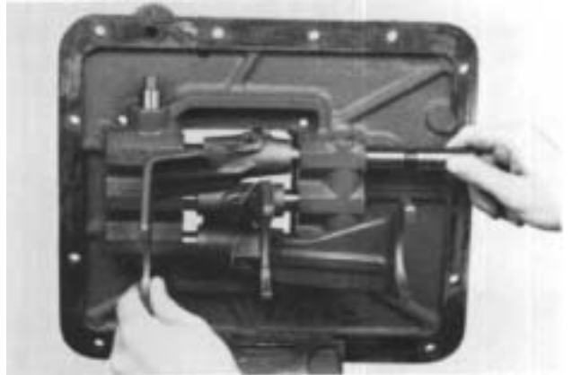
9. Install the 1st-reverse shift bar and yoke. Install the yoke lockscrew and tighten and wire securely.
