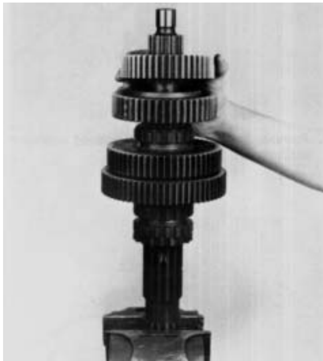
11. Remove the 4th speed gear and splined washer.
