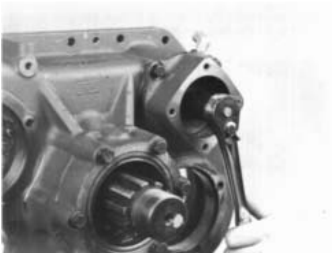
7. Install the locknut on the shaft.
