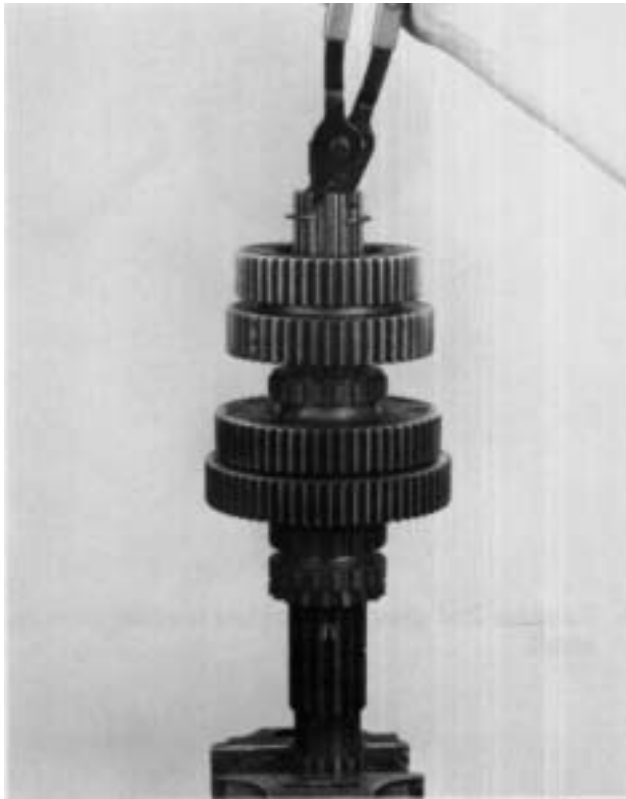
10. Remove the snap ring from the groove in the hub of the 4th speed gear.
