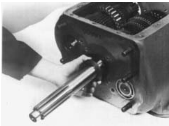
6. Install the spacer on the shaft, flat side of spacer against the gear, K 023
