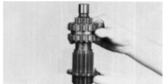
18. Remove the reverse gear splined washer and the 1st-reverse sliding clutch.
