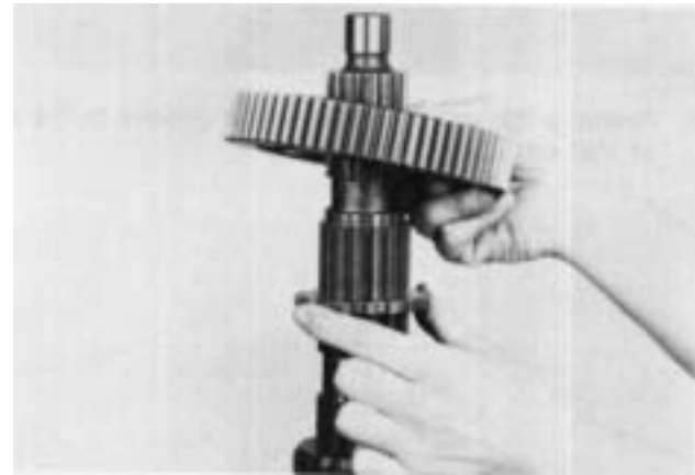
17. Remove 1st speed gear and splined washer from mainshaft.
