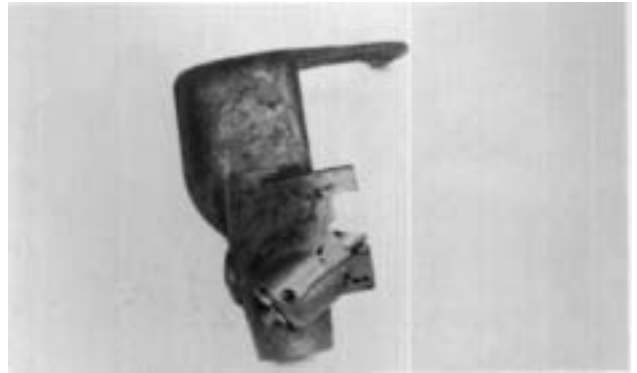
8. Partially install the plug. Use the tip of the gear shift lever to push the plunger back into the bore to compress the spring. Tighten the plug fully and then back off 1/2 - 1 1/2 turns. Stake the plug threads in the hole.
