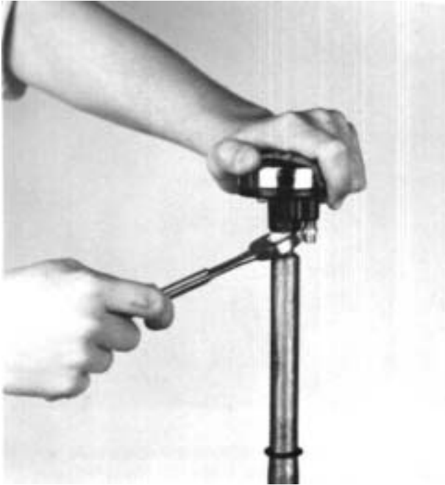
9. Loosen the jam nut and turn the nut and selector valve from the shift lever. Remove the air lines, sheathing and O-rings from the lever.
