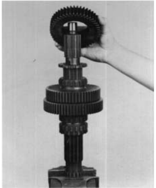
12. Remove the 3rd speed gear.
