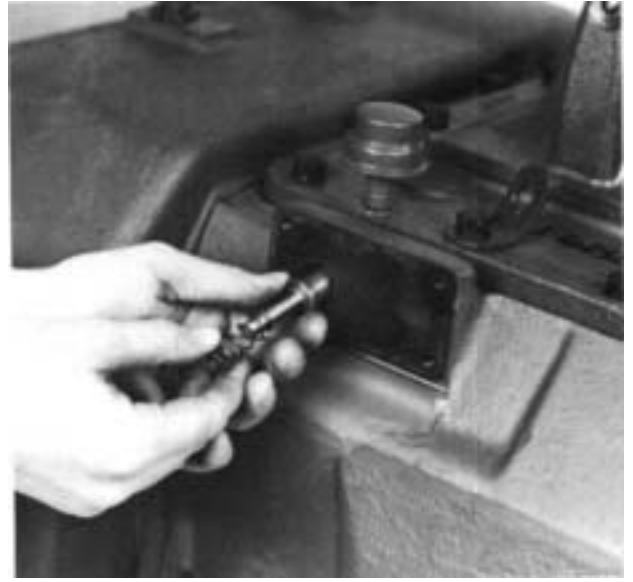
17. Remove the spring and plunger from the bore in the transmission.
