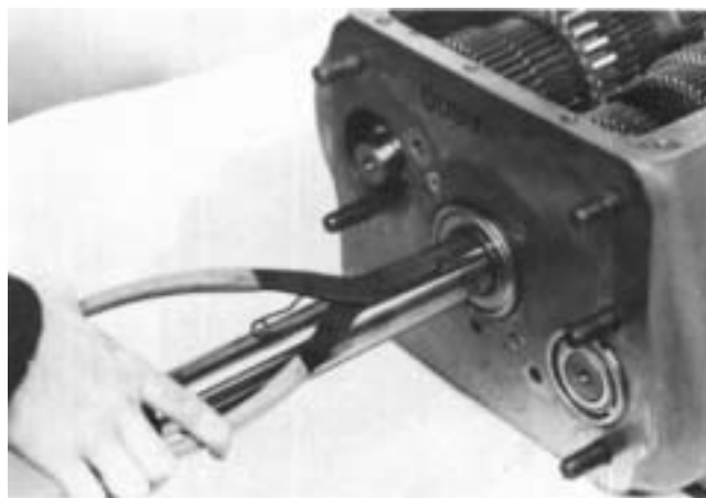
8. Install the snap ring in the groove of input shaft, with flat side of
