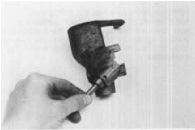
6. If previously removed, install the reverse-top plunger in the reverse yoke. Make sure that the plunger is fully seated in the bore.
