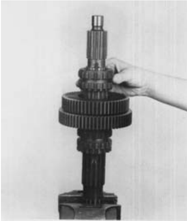
14. Remove the 2nd-3rd speed sliding clutch.
