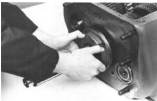
9. Align oil return slot of front bearing cover with oil return hole in front case and install bearing cover. Install 4 bearing cover retaining cap screws.
