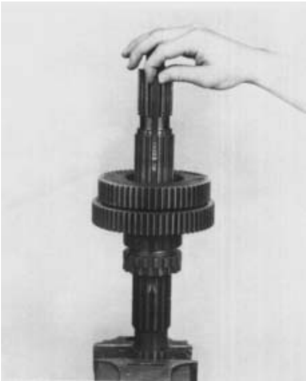
15. Remove the key from the mainshaft
