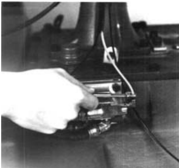
6. Disconnect the white 1/8" O.D. supply line at the forward "S" port of the slave valve.
