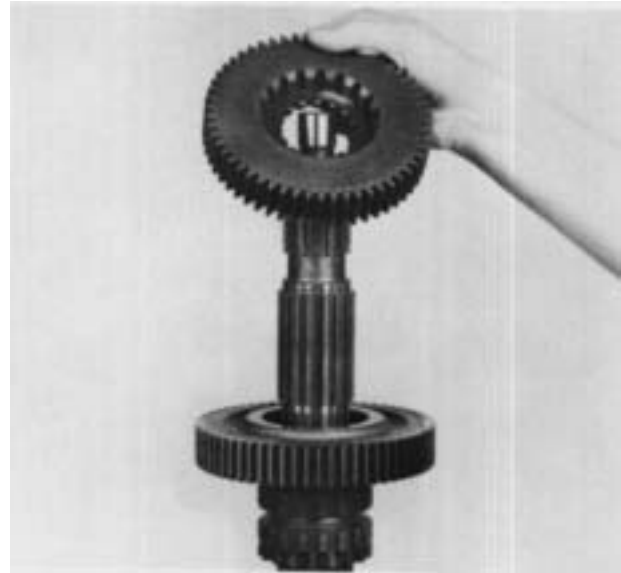
16. Remove 2nd gear and splined washer from mainshaft.
