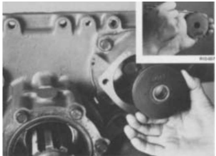
6. Remove the range piston from cylinder bore. If necessary, remove the O-rings from piston I.D. and O.D. (inset).
