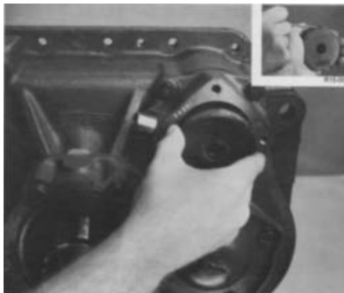
6. Remove the range piston from cylinder bore. If necessary, remove the O-rings from piston I.D. and O.D. (inset).
