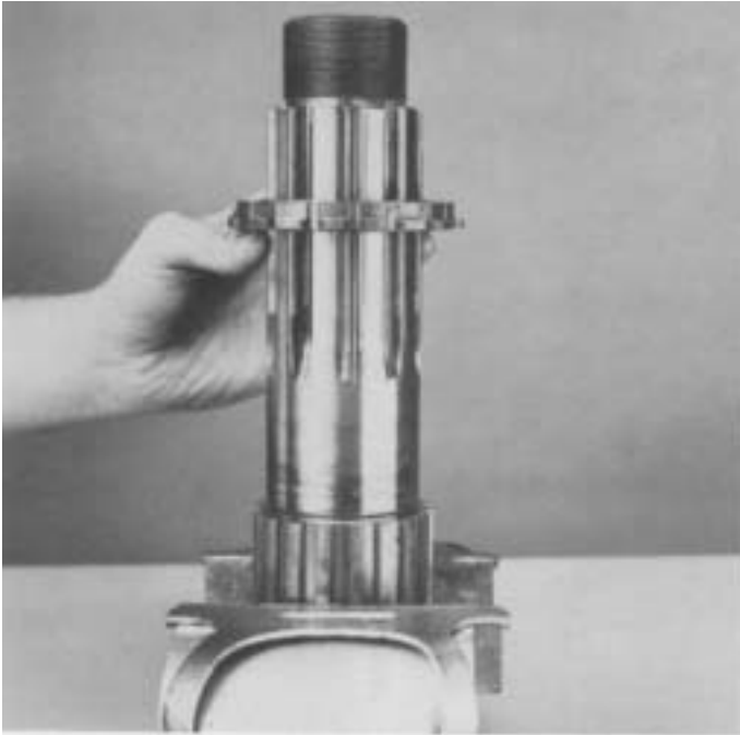
5. Remove the splined spacer from output shaft.
