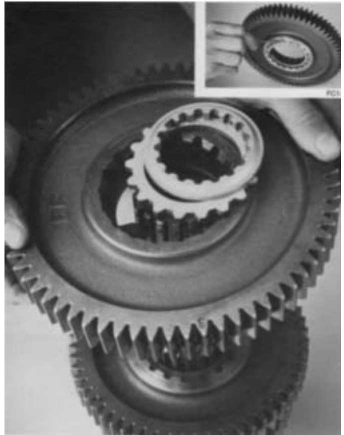
9. Pull the 1st speed gear from rear of mainshaft to remove limit washer, spacer and gear. If necessary, remove the snap ring from I.D. of gear (inset).
