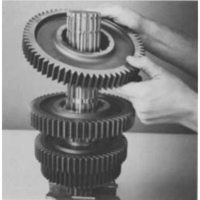
14. Install the 1st speed gear on shaft against 2nd speed gear, clutching teeth up.
