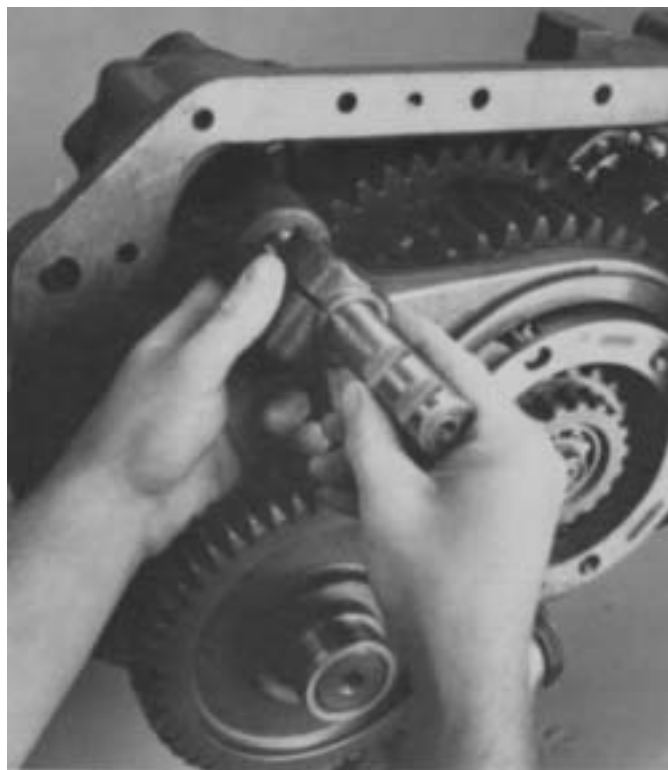
4. Pull yoke bar from bore of cylinder housing.
