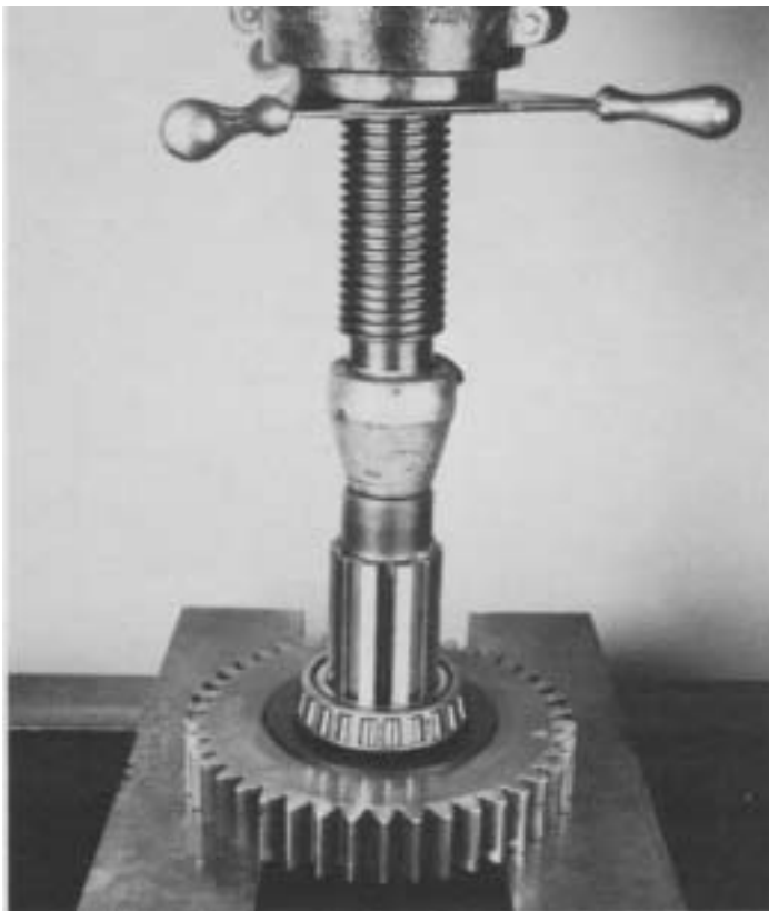
8. Using the front face of deep reduction gear as a base, press the output shaft through the bearing and gear. This will free the bearing, gear, washer, and, for models so equipped, the spacer or oil retention ring. DO NOT DAMAGE MAINSHAF 85 QUILL.
