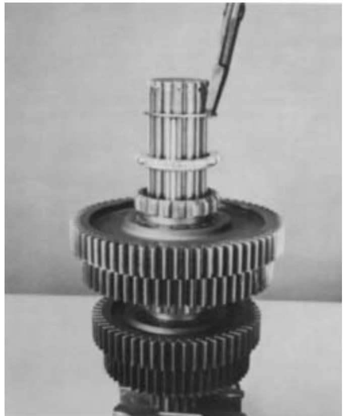
21. Install the snap ring in 6th groove of mainshaft to retain key in keyway.
