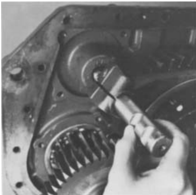
4. Pull yoke bar from bore of cylinder housing.
