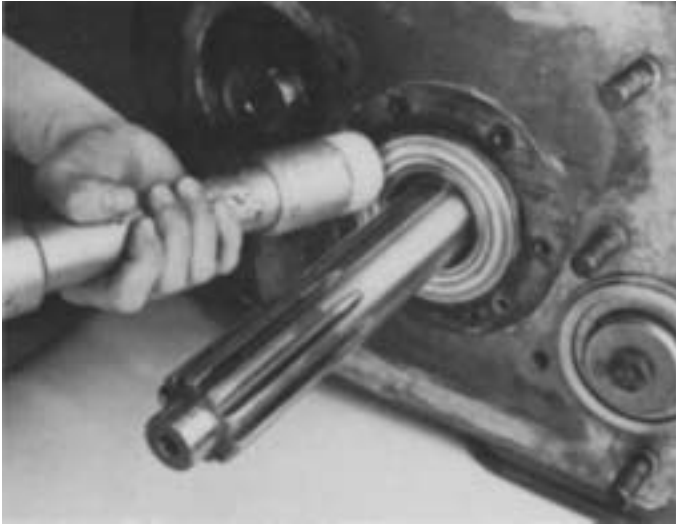
5. Tap the bearing into position in the bore with a soft mallet.
