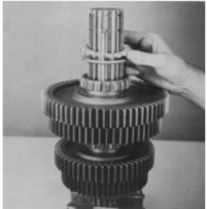
20. Install the spacer on shaft against washer.
