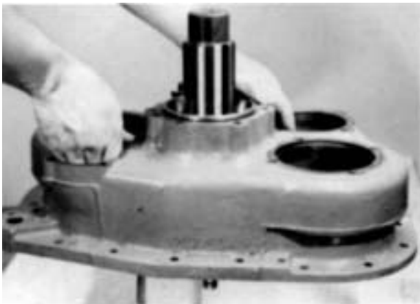
9. Place the housing over the output shaft, seating the bearing in the cup.
