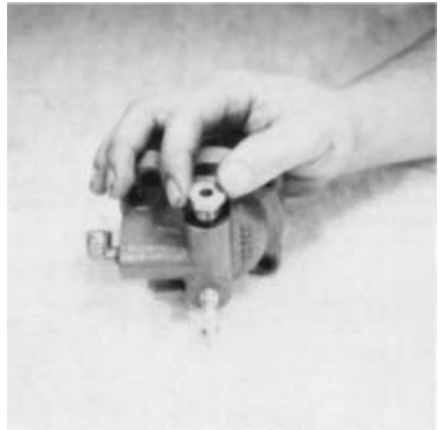
9. Install the exhaust screw in the cover to retain the insert valve.
