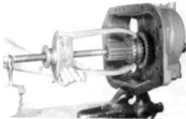
2. Use a puller on the sliding clutch to remove the mainshaft and clutch from the output shaft quill.
