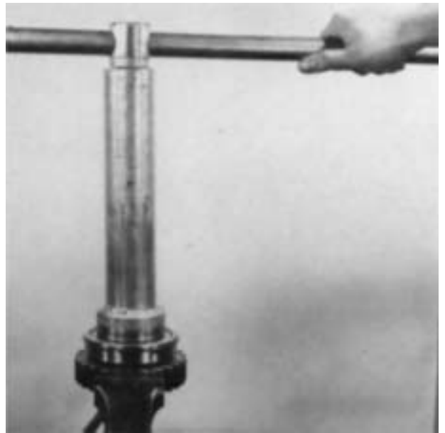
3. Relieve the bearing nut where it is peened into the shaft and turn the bearing nut from the shaft; left hand thread.
