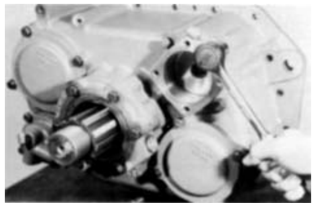
4. Remove the shift yoke, turn out the four capscrews and remove the cylinder housing from the auxiliary housing. If necessary, remove the O-ring from the bore in the cylinder housing.
