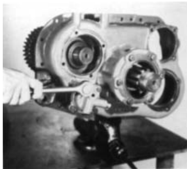
2. Remove the cylinder cover. If necessary, turn out the plug on the cover and remove the insert valve.
