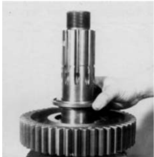
5. Install the washer on the shaft and against the gear with the side with the large groove facing up.
