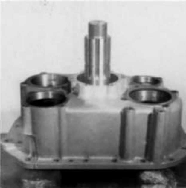
7. Install the rear housing over the output shaft, allowing the housing to rest on the reduction gear.
