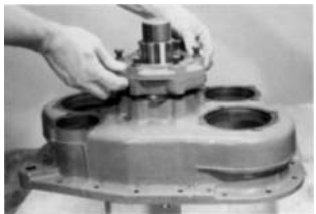
12. Install the bearing housing and gasket on the auxiliary housing; use a brass washer on the cap screw which passes through the speedometer bore.
