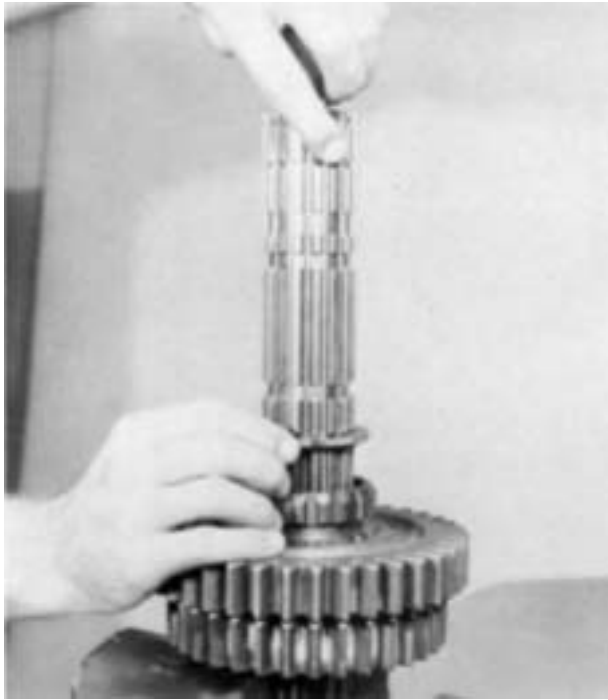
9. Remove the key and install the Low Limit first speed gear washer, flat surface up. Re-install the key.
