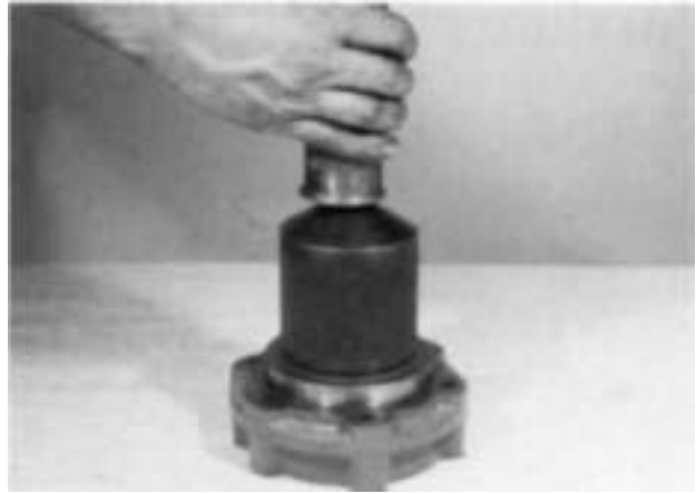
14. If previously removed, install the oil seal in the rear bearing housing with the seam to the inside. Use of a proper oil seal driver is recommended.
