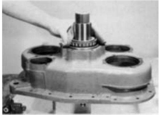
10. Heat the rear bearing cone and install on the shaft and in the cup. make sure that the lip of the cup is fully seated against the housing.
