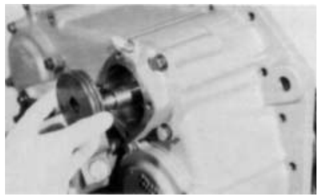
3. Remove the piston from the yoke bar and if necessary, remove the O-rings from the ID and OD of the piston. Push the yoke bar forward and from the housing.
