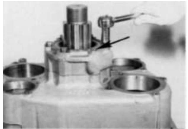
15. Install the rear bearing housing and gasket on the auxiliary housing, using a brass washer (arrow), at the speedometer bore. Make sure to match one of the notches in the surface of the bearing housing with the oil port in the auxiliary housing.
