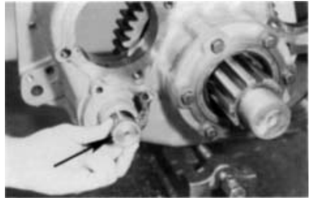
3. Push the yoke bar to the rear and remove from the housing. If necessary, remove the O-ring from the bar, (arrow).
