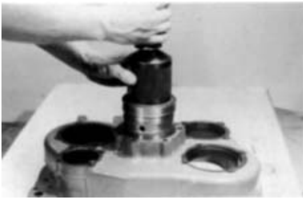
8. Start the front cup of the bearing into the auxiliary bore with the wide edge up. Stack the outer spacer and rear cup on the front cup and use a driver to seat all three evenly in the bore. Tap lightly to avoid driving the front cup out the bottom of the bore.
