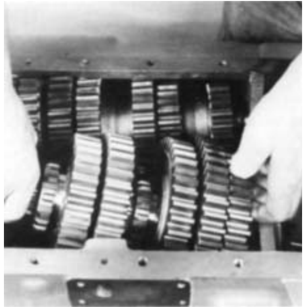
21. From inside the case, insert the rear of the mainshaft through the rear bearing bore and lower the assembly into position. Block the right countershaft against the side of the case and move the mainshaft pilot forward to seat in the pocket of the drive gear shaft.
