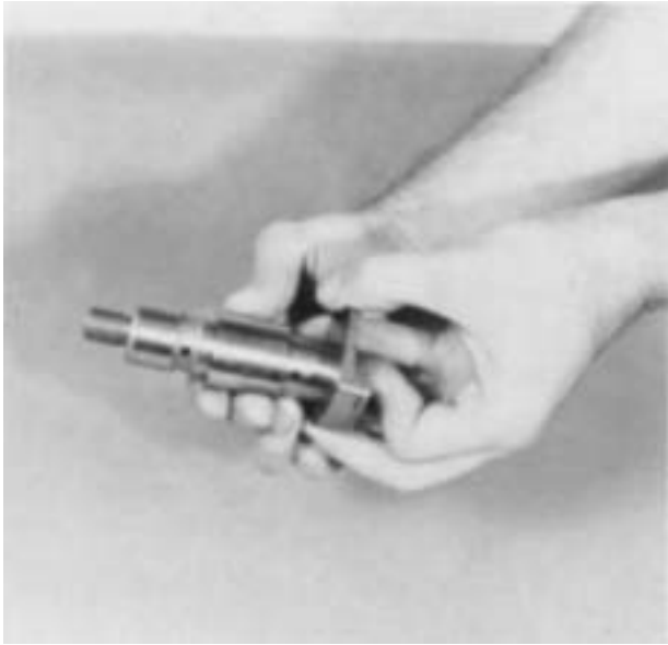
1. Install the plug in the end of the shaft and install the cup and bearing inner race on the shaft.
