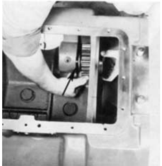
3. Install the gear and thrust washer on the shaft as the shaft is inserted into the bore. Make sure that the long hub of the gear (arrow), faces towards the front of the case.
