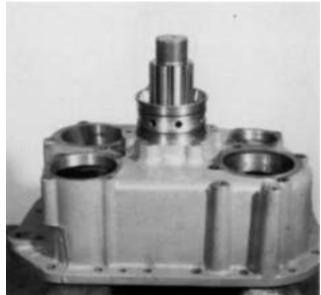
10. Stack the two bearing cups and outer spacer in the output shaft bore in the proper sequence. Make sure that the front bearing cup taper matches the taper direction of the front bearing cone.
