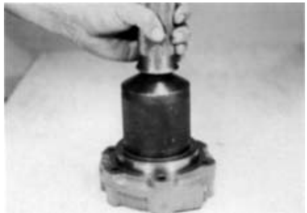
11. If previously removed, install the oil seal in the bearing housing with the surface with the seam to the inside.
