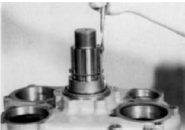
13. Install the speedometer drive gear or replacement spacer on the shaft and against the rear bearing cone and secure with the snap ring.
