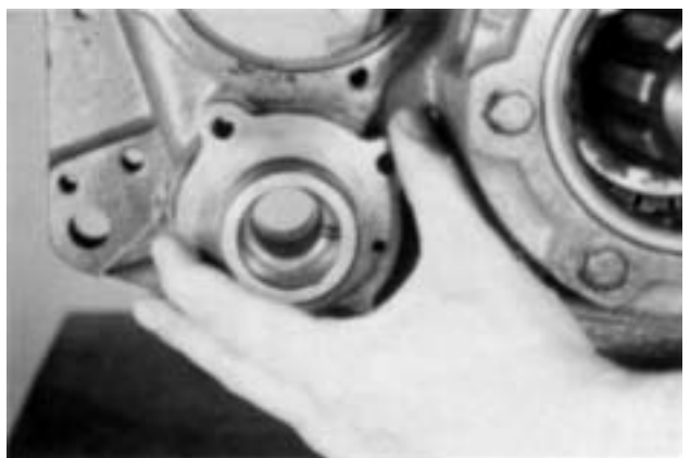
4. Remove the shift yoke and cylinder housing from the auxiliary housing. If necessary, remove the O-ring from the bore in the cylinder housing.
