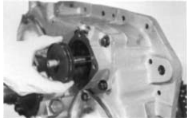
3. Remove the piston from the yoke bar and if necessary, remove the O-rings from the OD and ID of the piston. Push the yoke bar forward and from the housing.
