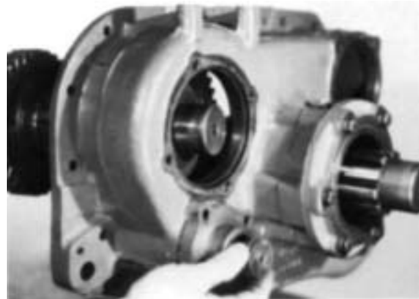
3. Pull the yoke bar from the cylinder housing; remove the O-ring if necessary.
