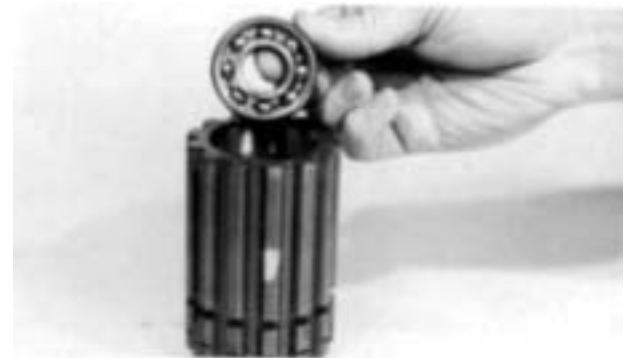
3. If necessary, remove the bearing from the mainshaft by tapping lightly from the inside with the range shift yoke bar or a similar size rod.
