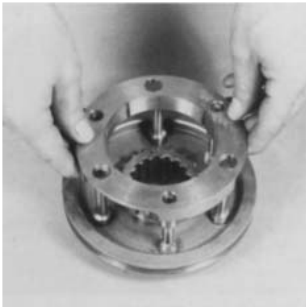
2. Pull the direct (high range) cone synchronizer from the pins of the low speed synchronizer ring. Cover the assembly with a cloth as the three springs will be released at the blocker pin locations.
