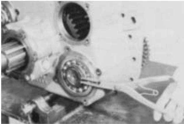
2. Remove the snap ring from the rear of each auxiliary countershaft.
