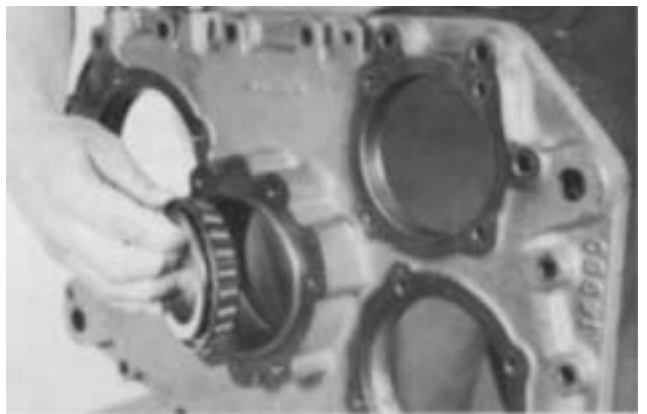
8. Remove the bearing rear cone from the housing.
