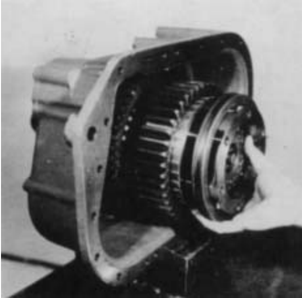
1. Pull the synchronizer assembly from the splines of the output shaft.
