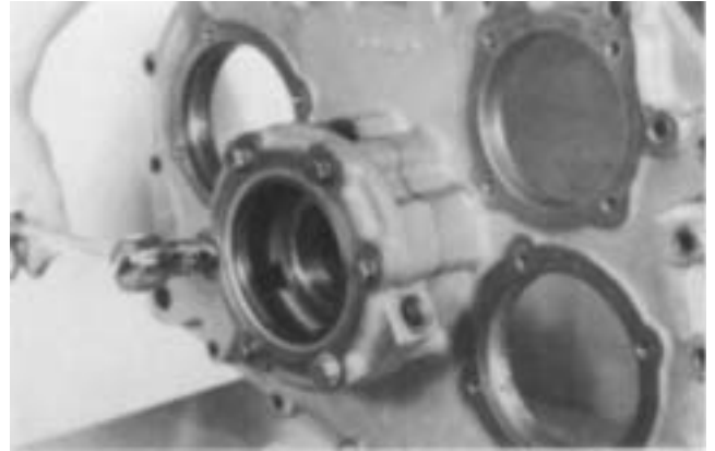
7. Turn out the cap screws and remove the rear bearing cover. If necessary, remove the oil seal from the cover.
