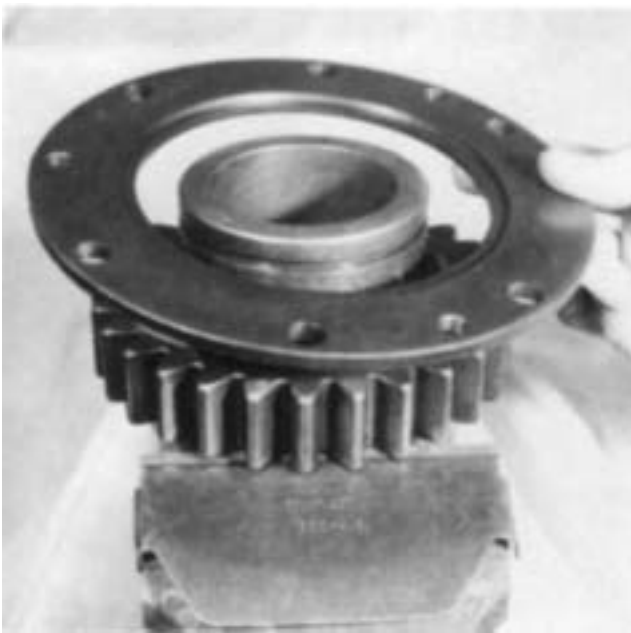
1. Install the retainer ring on the gear with the groove in the ring facing away from the gear.
