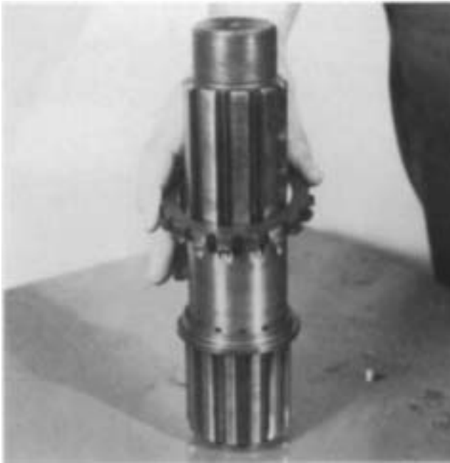
5. Remove the splined spacer from the shaft.
