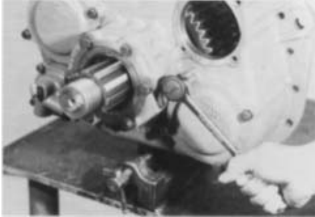
1. Turn out the capscrews and remove the two rear bearing covers.
