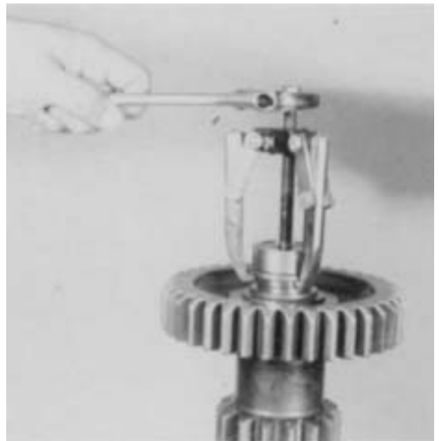
5. If necessary, remove the bearing inner race from the front of each countershaft with a puller or pry bars.
