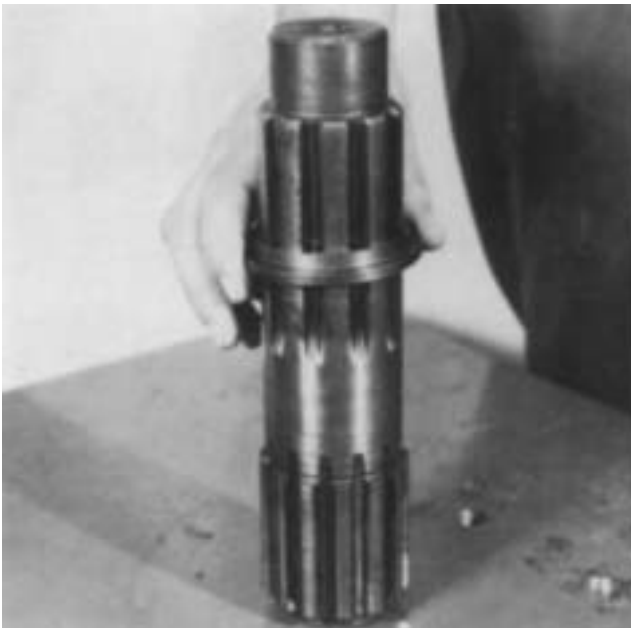
6. Remove the stepped washer from the shaft.
