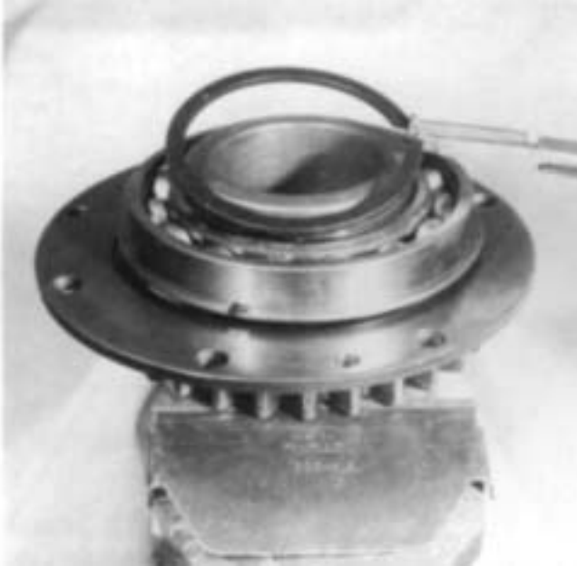
3. Install the snap ring in the drive gear groove to secure the bearing to the gear.
