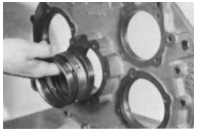
9. Remove the two bearing cups and outer spacer from the housing bore.
