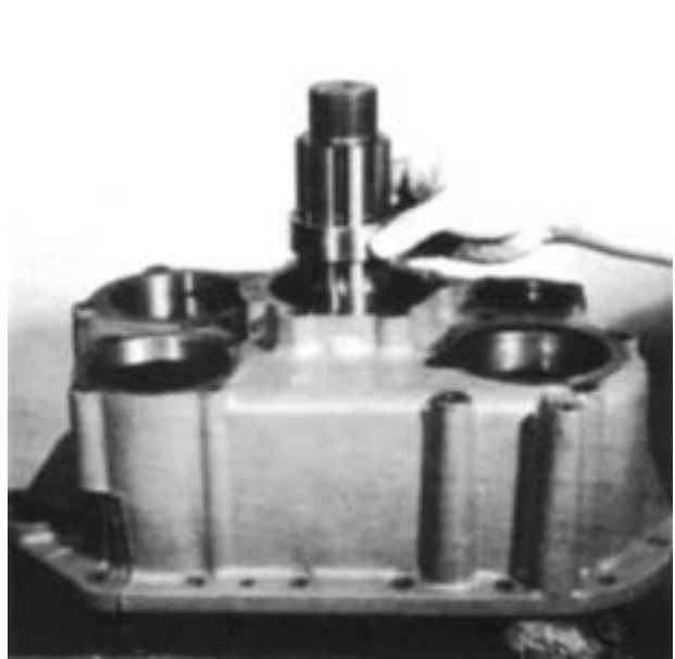
9. Install the bearing inner spacer on the shaft and against the front bearing cone.
