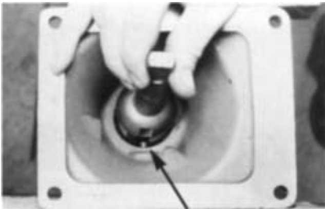
3. Install the housing in a soft-jawed vise with the bottom facing up and insert the shift lever in the housing, fitting the slot in the pivot ball of the lever with the pivot pin.
