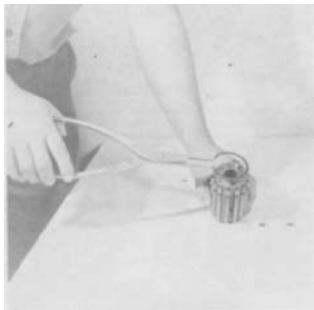
8. If necessary, remove the snap ring from the OD of the shaft. Check the bushing in the shaft and replace if worn.
