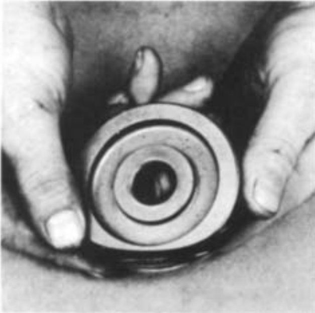
3. Install the O-rings in the O D and ID of the piston.
