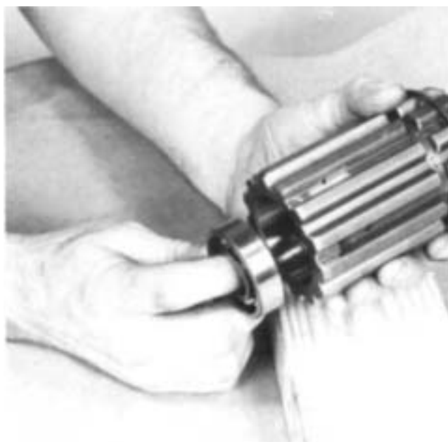
7. Remove the bearing from the shaft. If necessary, use an inside jaw impact puller.
