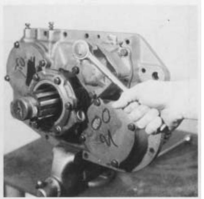
6. Install the shift cylinder cover on the housing with the air fitting to the top left.
