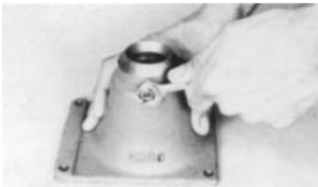
2. Install the pivot pin in the housing, threaded end out, and secure with the nut and lockwashers.
