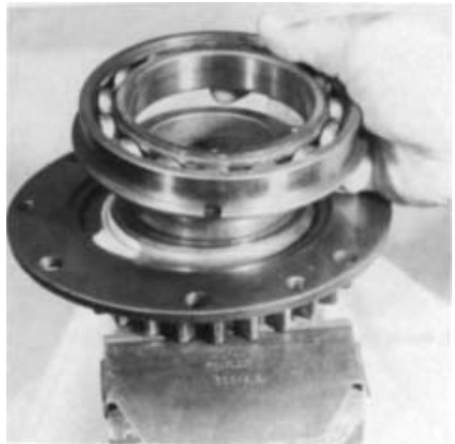
2. Install the bearing on the gear with the snap ring facing the groove in the retainer. Tap lightly on the inner race of the bearing with a soft bar and mall.
