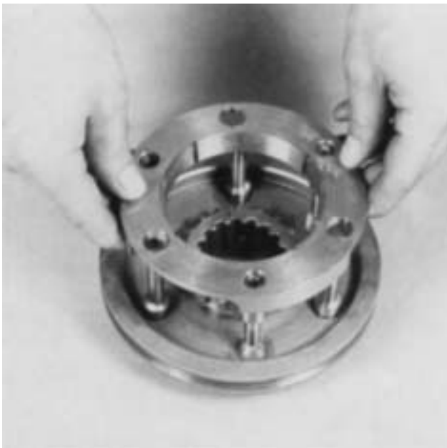
2. Pull the direct (high range) cone synchronizer from the pins of the low speed synchronizer ring. Cover with a cloth as the three springs will be released at the blocker pin locations.
