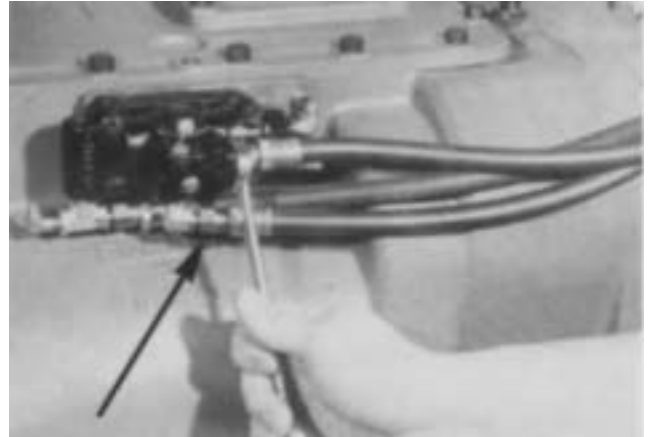
5. Remove the hose clamp and disconnect the two 1/4" ID air lines between the air valve and the range shift cylinder.
