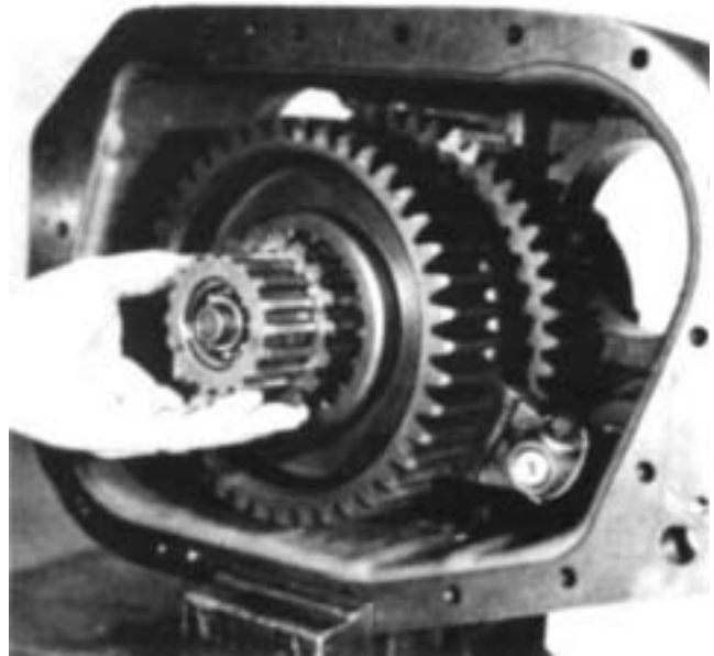
3. Install the splined washer on the shaft and in the hub of the gear. Turn the washer to lock the gear on the shaft.
