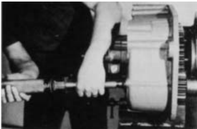
3. Use a soft bar and mallet to drive the countershaft forward and from the rear bearings.
