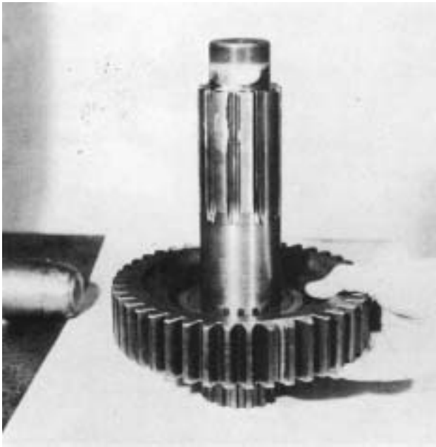
3. Install the low speed gear on the shaft with the clutching teeth down and engaging the splines of the spacer.
