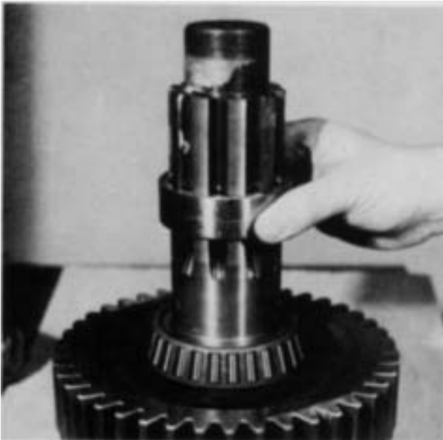
2. Remove the bearing inner spacer from the shaft.
