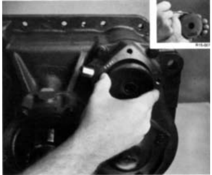
6. Remove the range piston from cylinder bore. If necessary, remove the O-rings from piston I.D. and O.D. (inset).
