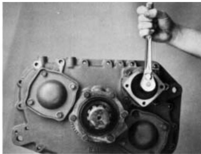
2. Remove nut from end of yoke bar.
