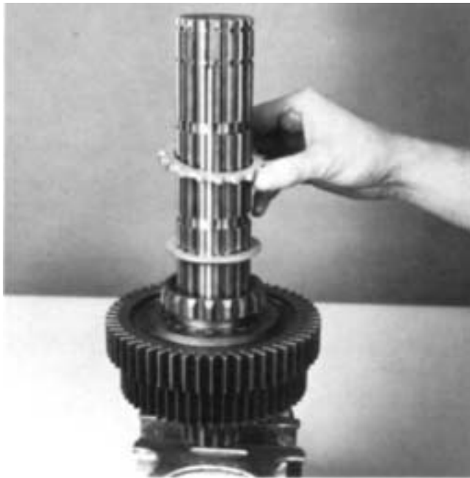
12. Install the spacer on shaft against washer.
