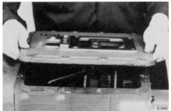
2. Jar to break the gasket seal and lift the shift bar housing from transmission.
