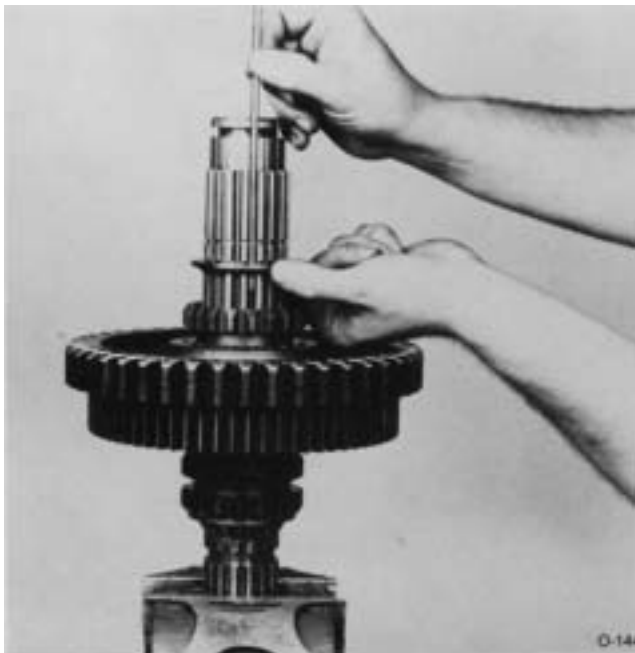
13. Remove key and install reverse gear limit washer, flat side up, in last groove of mainshaft. Rotate washer to align splines of washer with those of mainshaft and reinsert key.
