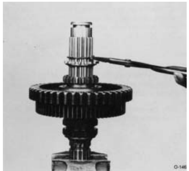
15. Install snap ring in snap ring groove at rear of mainshaft.
