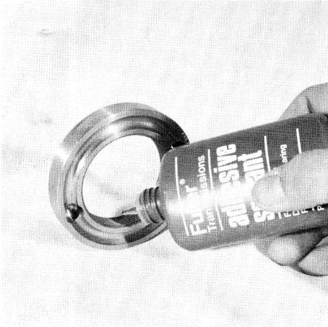
5. Apply Loctite, grade AVV, to the threads of the drive gear nut. The threads must be dry and free from dirt and grease.
