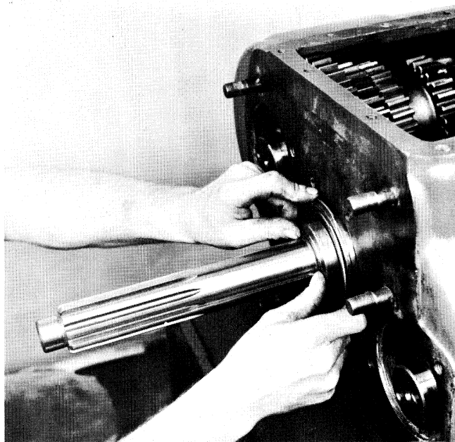
10. Install the snap ring in the groove in the bearing.
