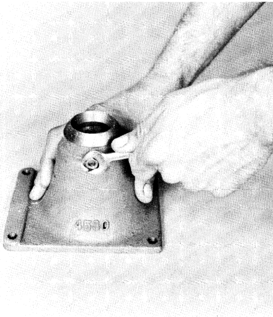
2. Install the nut, pivot pin and washer in the side of the housing, pin to the inside.
