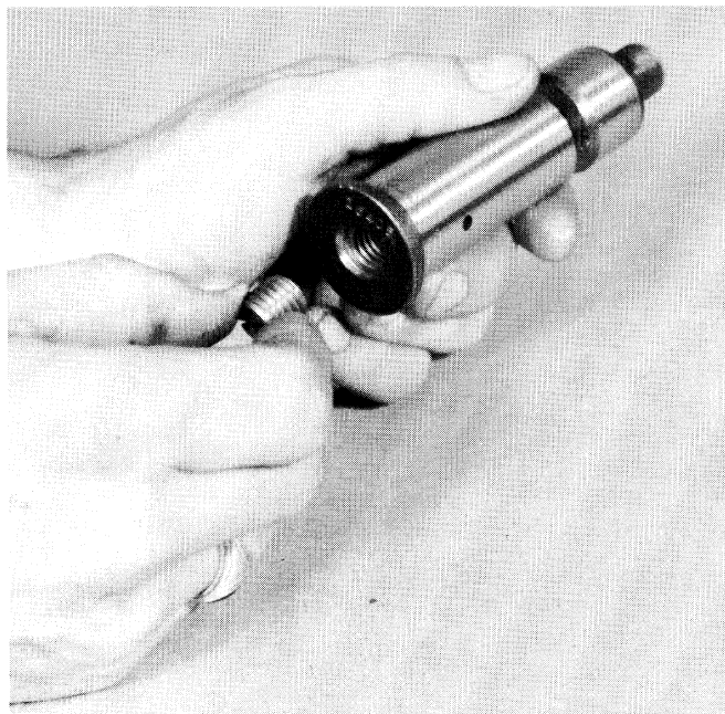
1. Install the plug in the idler shaft.
