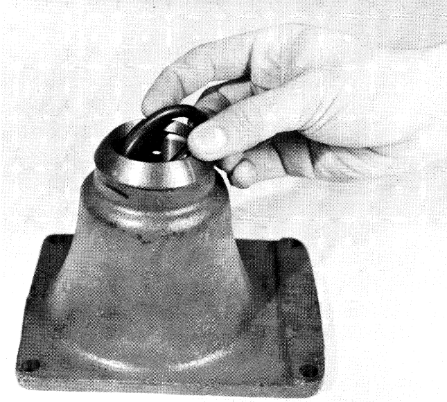
1. Install the O-ring in the groove at the top of the gear shift lever housing.
